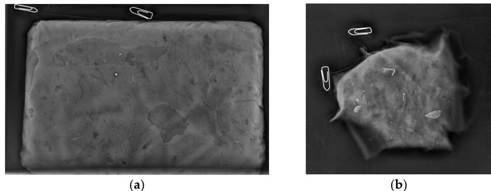
**Figure 2.** X-ray of packages containing minced meat from wild game that had tested negative for metal parts by the metal detector. (a) Near to the center, a metal-dense object of ca. 1.5 mm diameter (Pb content < 1.5 mg/kg); (b) one object of <1 mm diameter, smaller dense objects (Pb content = 57.1 mg/kg) and larger bone fragments.
