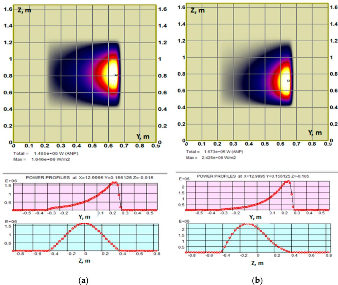
**Figure 14.** BTR plots with NB shine-through PD at FNS-ST first wall (NBI port size  $0.3 \times 0.6$  m<sup>2</sup>) for two operation cases: (a) ideal beam focus, total power—0.147 MW, peak PD—1.65 MW/m<sup>2</sup>; (b) beam misalignment  $4/-6$  mrad in horizontal and vertical planes, total power—0.167 MW, peak PD—2.43 MW/m<sup>2</sup>.
