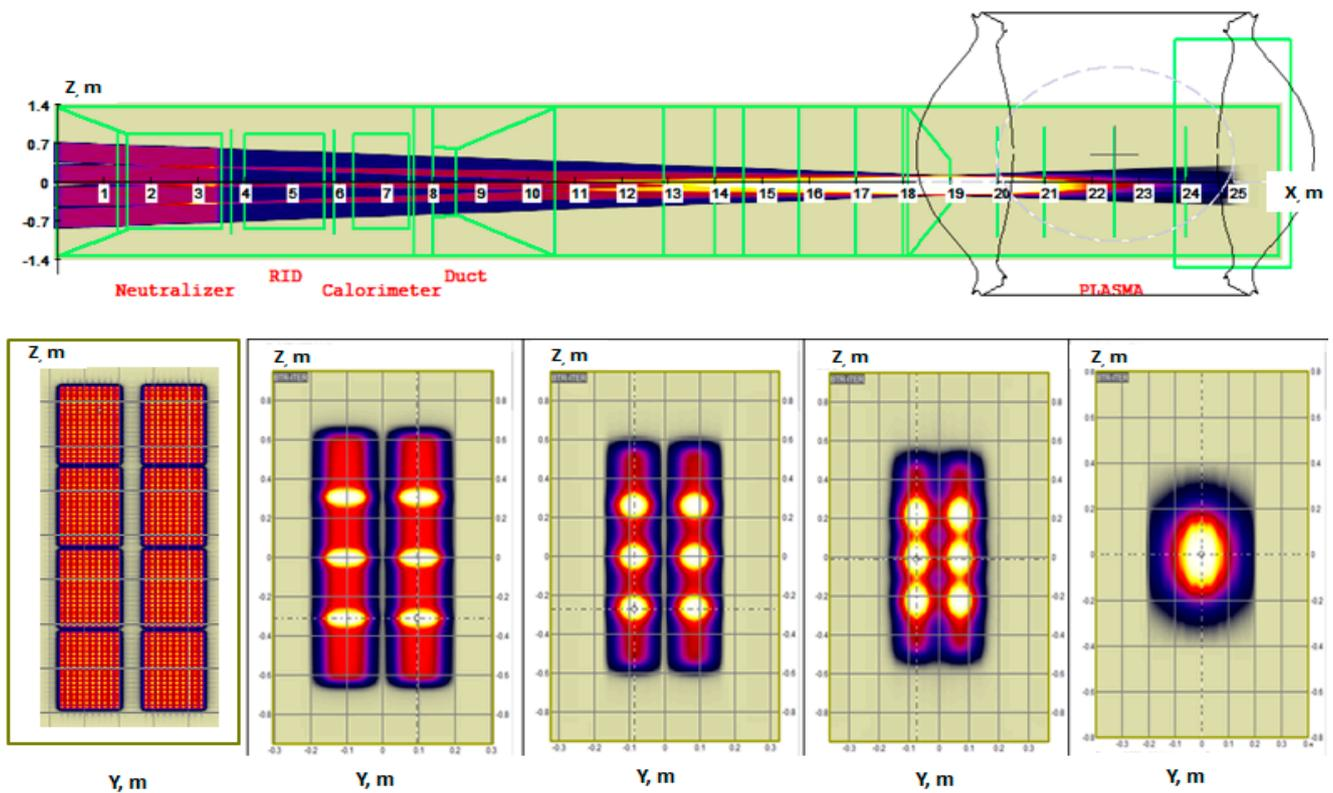
Figure 7. BTR plots with neutral beam power density at virtual planes: upper—along the beamline; lower—across the beamline (taken at different distances from BS GG).
