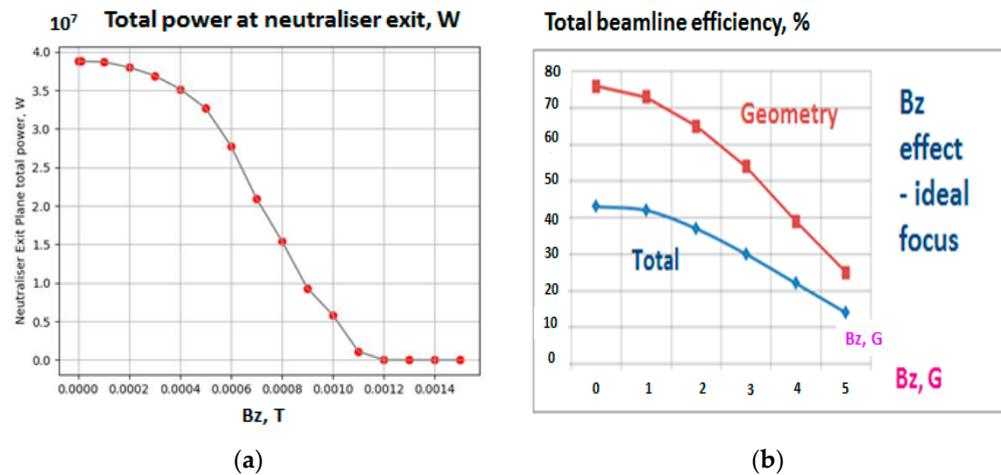
Figure 15. DEMO-FNS NBI efficiency as a function of vertical magnetic field ( $B_z$ ): (a) total neutral power ( $P_{Neutr}$ ) at the Neutralizer exit; (b) beamline geometry transmission ( $P_{inj}/P_{Neutr}$ ) and total power efficiency ( $P_{inj}/P_0$ ) shown in %.
