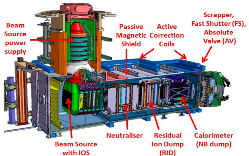
Figure 1. Neutral beamline without transmission ducts.
