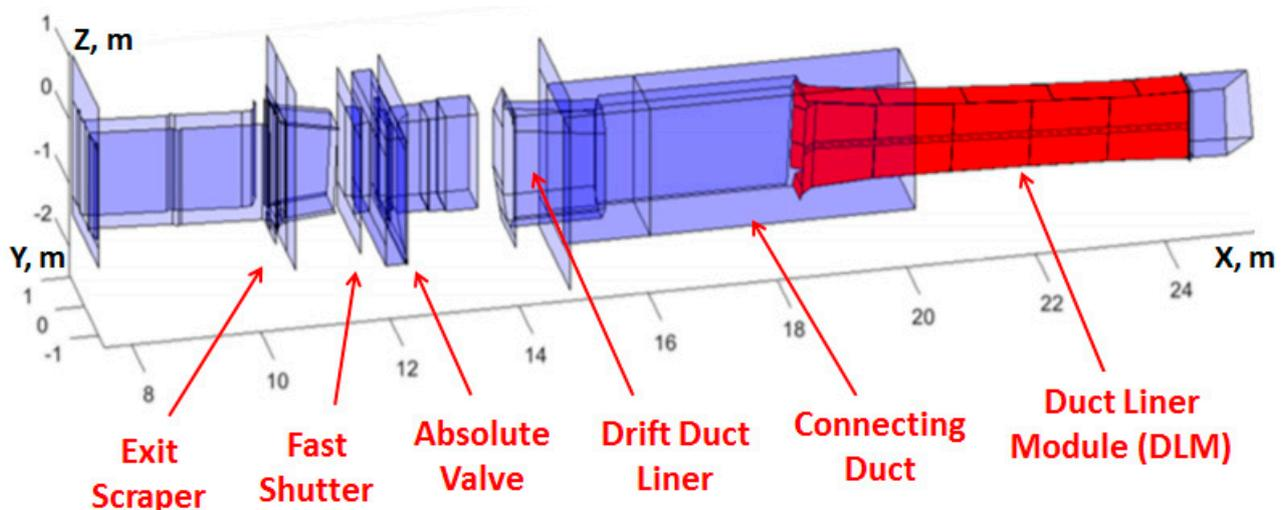
Figure 2. Outline of NBI transmission ducts (import from CAD).
