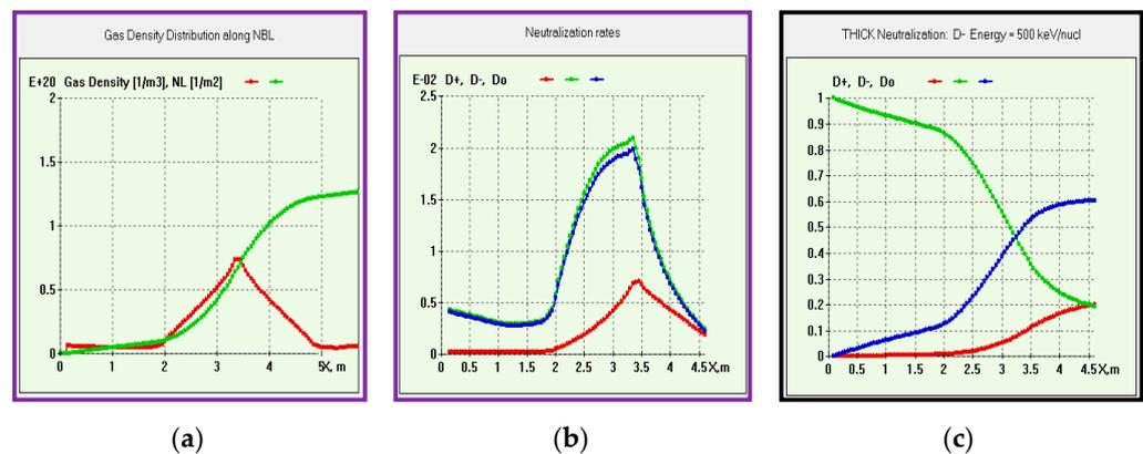
**Figure 9.** BTR subplots with gas target and beam fractions in the neutralizer (ITER NBI): (a) gas local density and thickness; (b) species source/loss rates; (c) species integral output.
