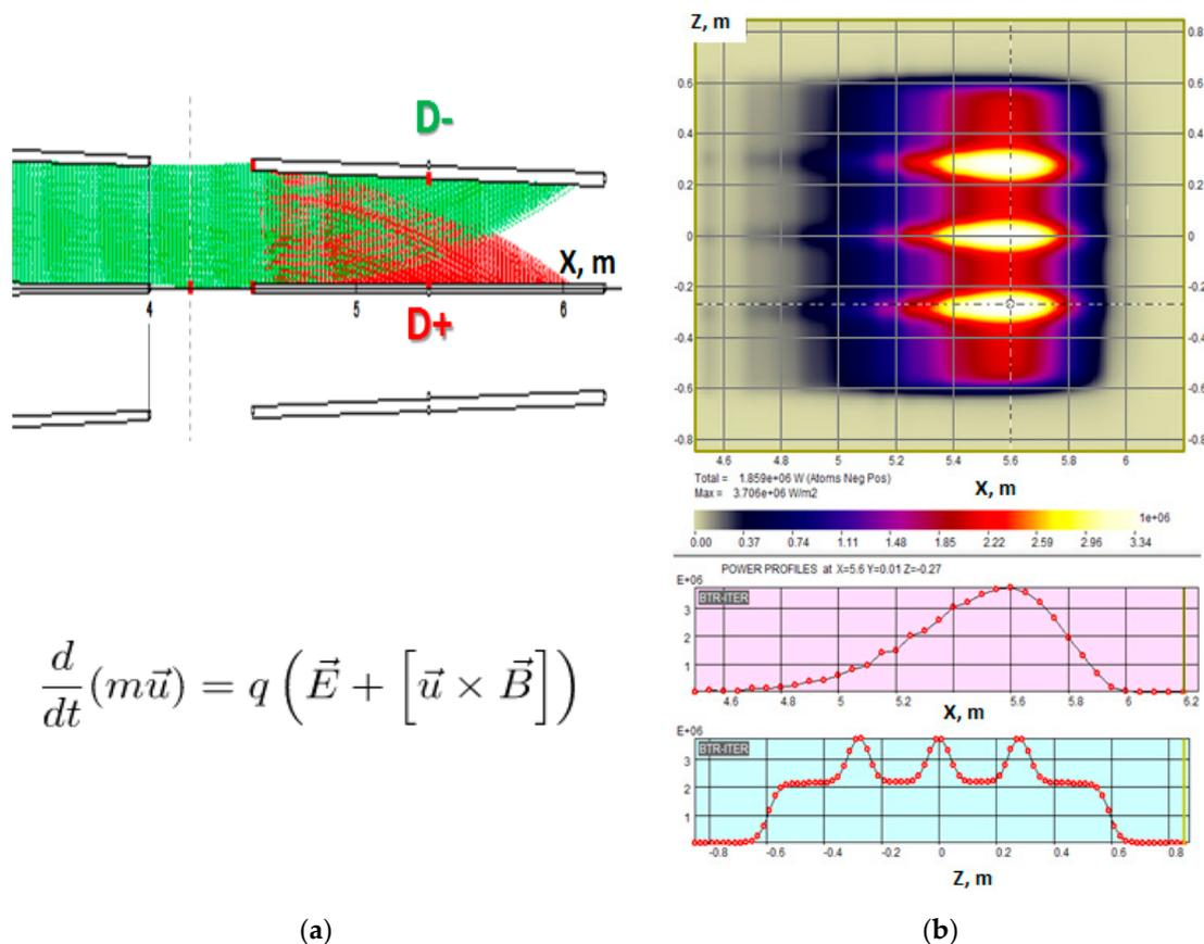
**Figure 10.** Residual ions deflection and dumping in ERID channel (DEMO-FNS): (a) positive/negative ions trajectories; (b) power density map and profiles at the dumping panel.
