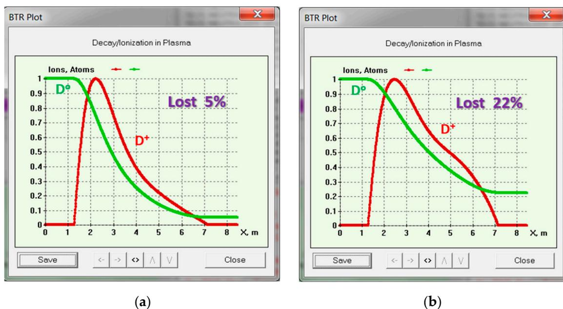
**Figure 19.** BTR plots with injected neutral beam stopping in DEMO-FNS tokamak for two values of plasma density: (a)  $n_e = 10^{20} \text{ m}^{-3}$ ; (b)  $n_e = 0.5 \times 10^{20} \text{ m}^{-3}$ .
