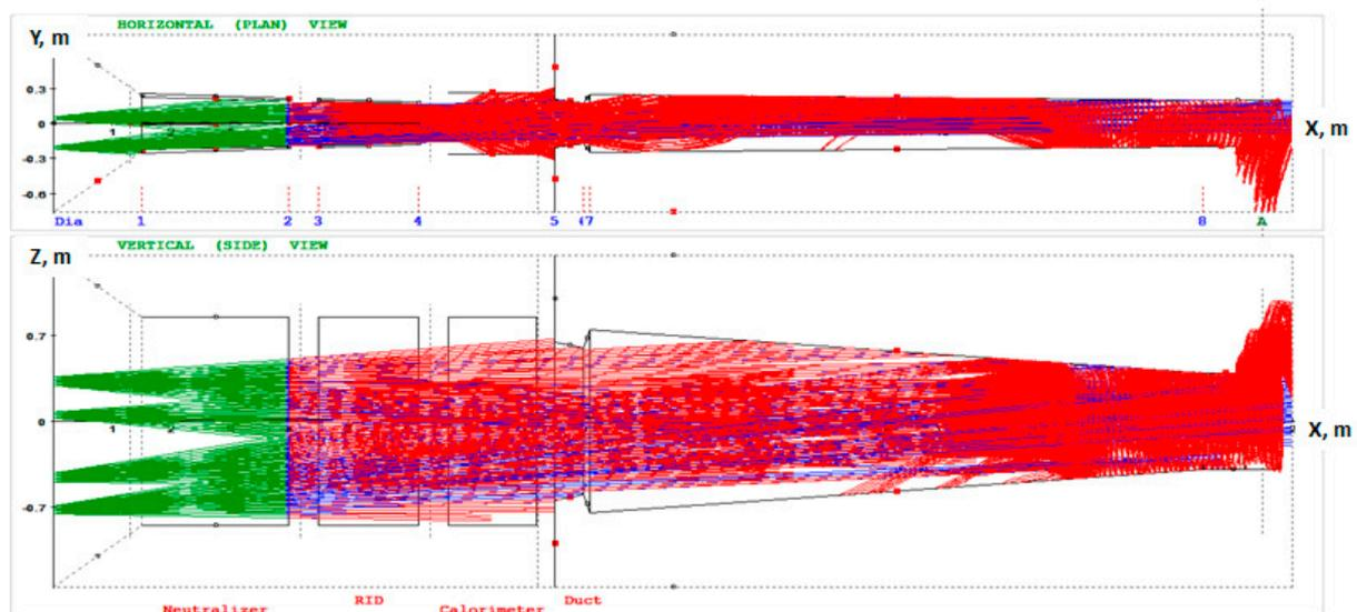
**Figure 11.** BTR screen with re-ionized particles (red) downstream of the neutralizer (DEMO-FNS). Atoms are shown in blue, negative source ions—in green color.
