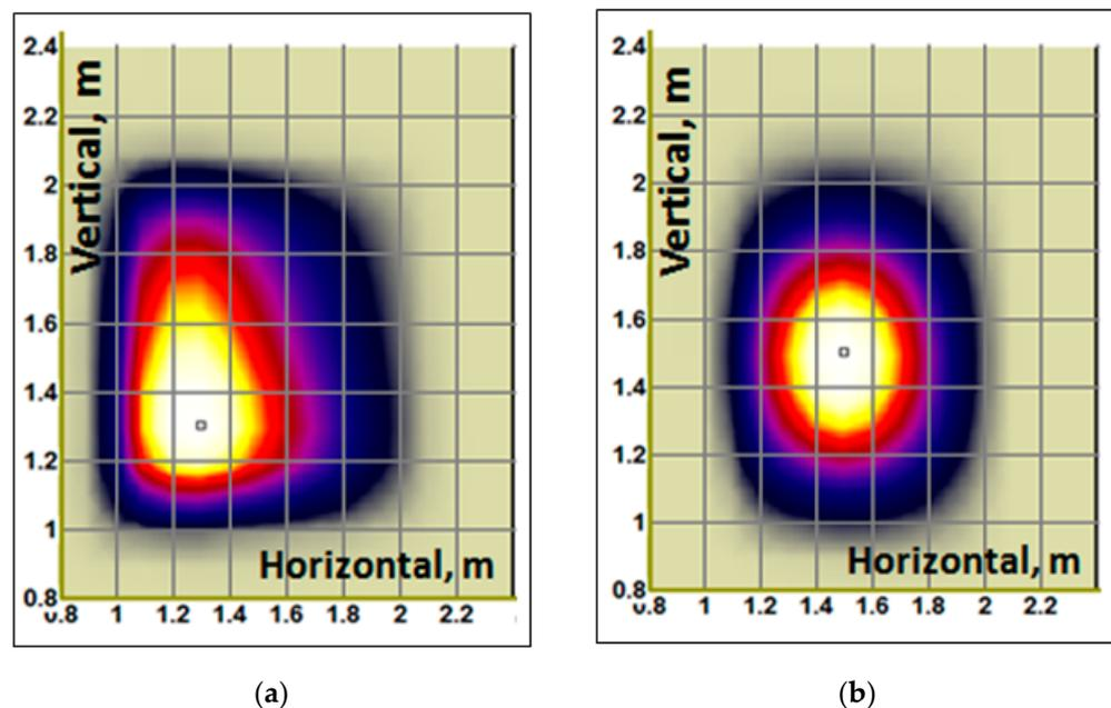
**Figure 20.** BTR plots with the injected neutral beam shine-through power footprints at the first wall in DEMO-FNS tokamak: (a) rectangular beam shape; (b) gauss beam shape.
