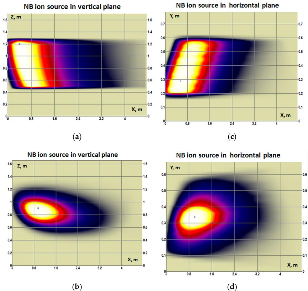
**Figure 13.** BTR subplots with neutral beam spatial deposition (ionization rate intensity) in DEMO-FNS plasma (BTR plots) along the injected neutral beam axis (NB enters from the left): (a,b) vertical cross-section plane, (c,d) horizontal cross-section plane; (a,c) correspond to rectangular beam shape; (b,d) refer to the realistic beam shape—with divergence and beamlet focusing.
