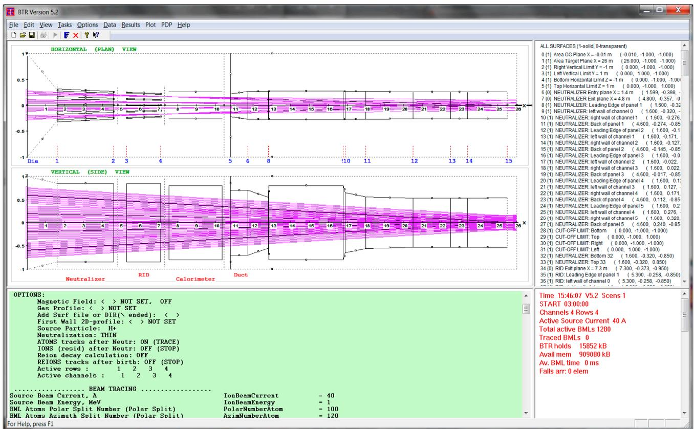
**Figure 5.** BTR screen with beamline standard ITER-like geometry and beamlets' axes (X, Y, and Z units are [m]).
