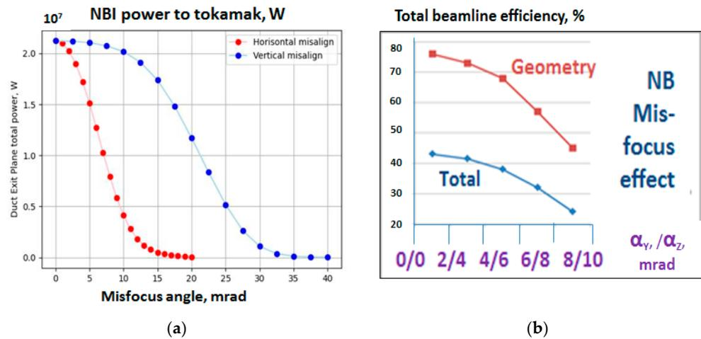
Figure 16. DEMO-FNS NBI efficiency as a function of beam misalignment in horizontal and vertical planes: (a) total injected power ( $P_{inj}$ ) at the duct exit; (b) beamline geometry transmission ( $P_{inj}/P_{Neutr}$ ) and total power efficiency ( $P_{inj}/P_0$ ).
