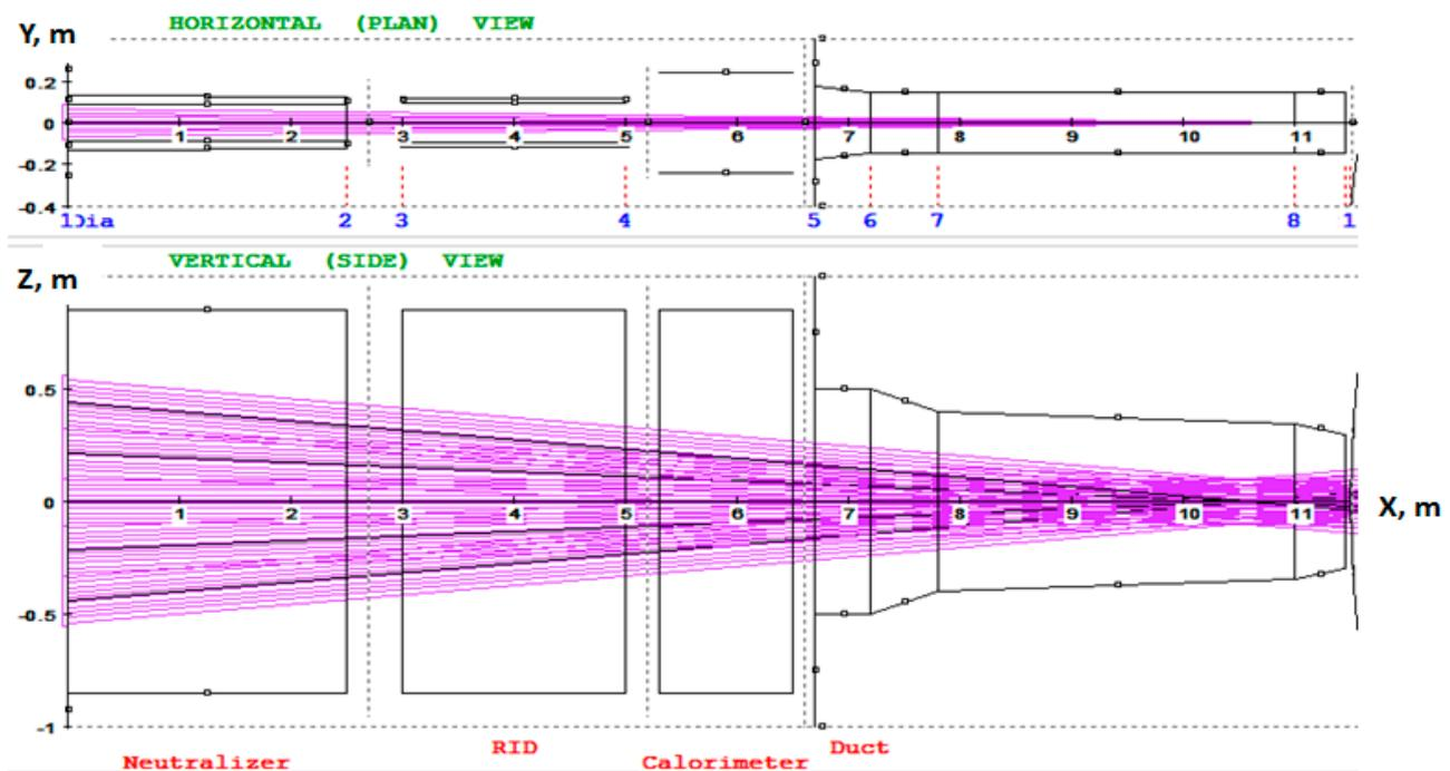
**Figure 3.** NBI beamlets axes focusing in FNS-ST compact NBI model.
