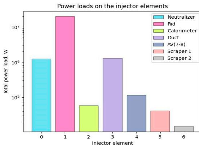
**Figure 17.** Total power deposition at DEMO-FNS NBI major components during the beam injection to tokamak (with calorimeter in open position).
