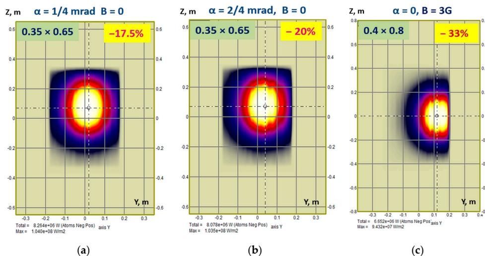
**Figure 18.** BTR subplots showing the injected beam footprints in NB port plane illustrating the effect of the beam misfocusing and/or magnetic field on injected beam power in DEMO-FNS tokamak: (a) source beam misalignment values in horizontal and vertical directions 1 mrad and 4 mrad (17.5% lost); (b) misalignment values 2 mrad and 4 mrad (20% lost); (c) ideal beam focusing with vertical magnetic field 3 G (33% lost).
