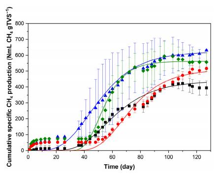
**Figure 1.** Adjustment to the experimental values of the cumulative  $CH_4$  production of each test under thermophilic conditions (55 °C) to the modified Gompertz model:  $\blacksquare$  Microcrystalline cellulose; • 1G vinasse;  $\blacktriangle$  2G vinasse;  $\blacklozenge$  co-substrate.
