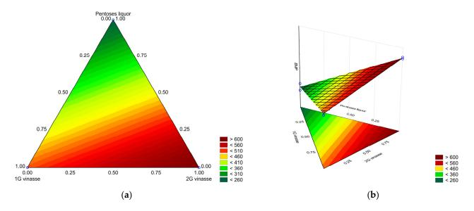
**Figure 2.** Fitted surface of the blend gradient of the substrates for specific CH<sub>4</sub> production: (**a**) 2D; (**b**) 3D.
