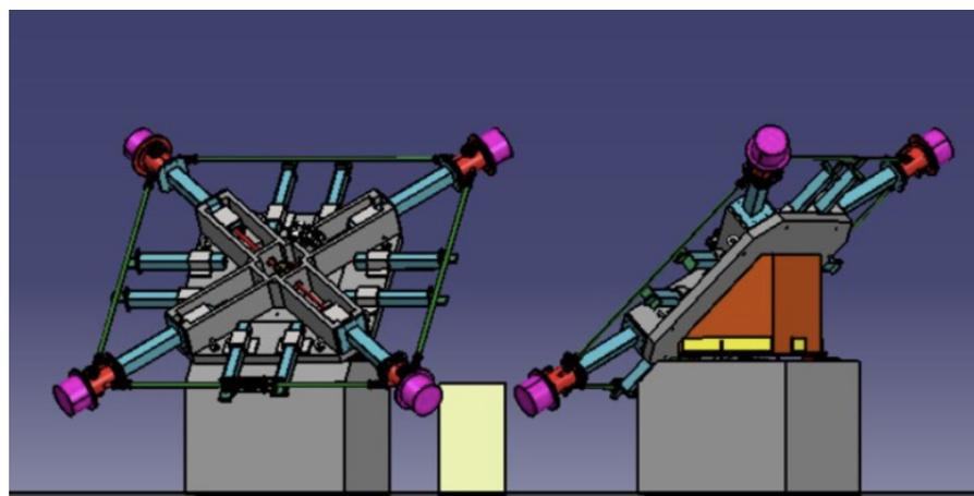
**Figure 2.** Pictorial view of GINGER, the two RLGs are visible. Compared to the previous project, sections and orientation have been changed.
