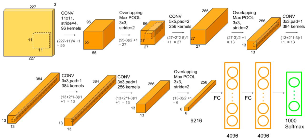
**Figure 8.** Pre-trained AlexNet CNN architecture [66].
