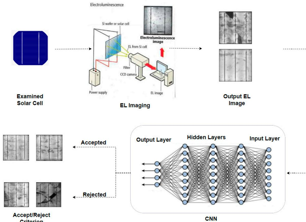
**Figure 1.** Summary of CNN-based identification of PV cracks.
