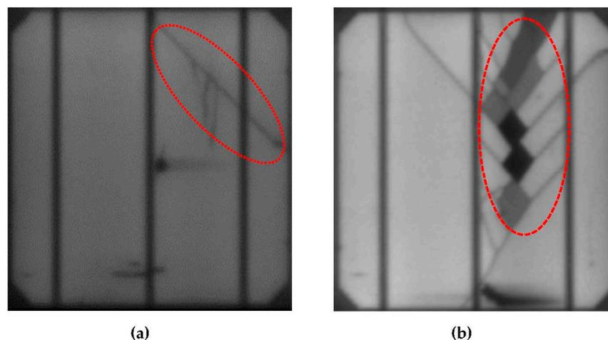
**Figure 2.** An EL image of a cracked solar cell (a) Mini-crack; (b) Major-crack.
