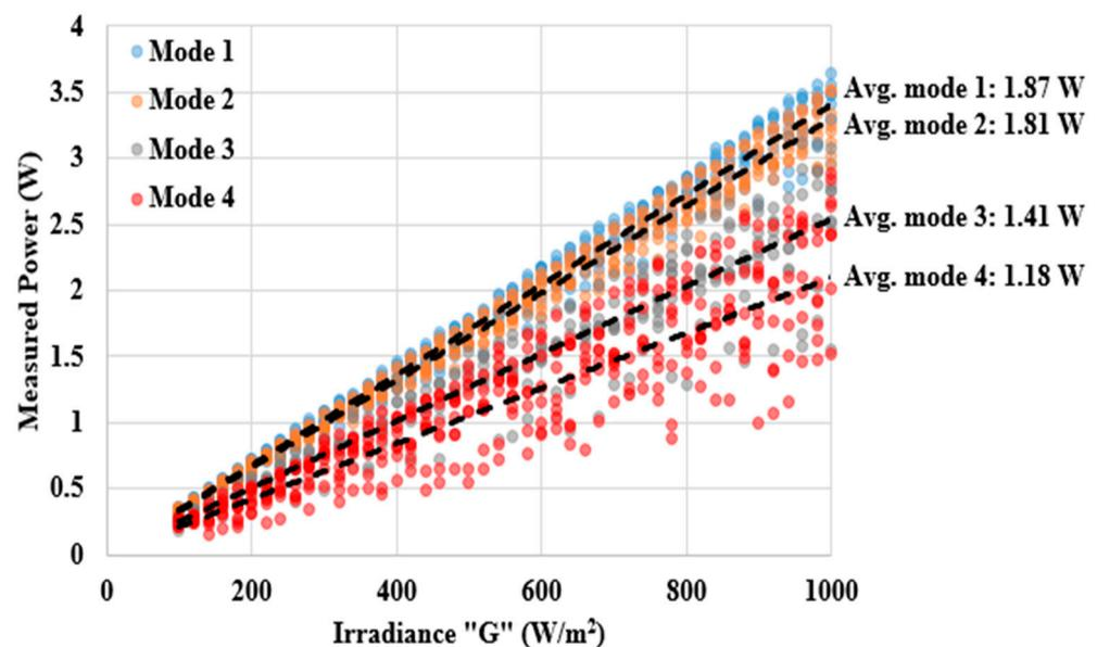
Figure 3. Measured power vs irradiance of the examined solar cells [22].
