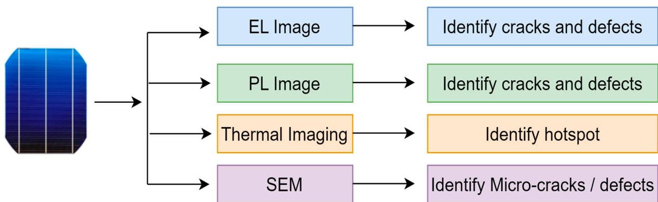
**Figure 5.** Different methods of detecting solar cell defects.
