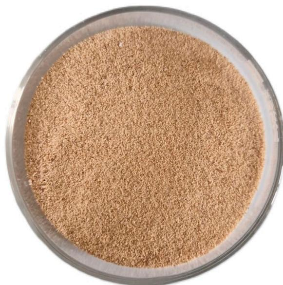
**Figure 1.** The vegetable filler used in this study: olive pit powder.
