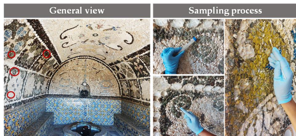
**Figure 1.** Casa de Fresco located in Condes de Basto Palace (Évora, Portugal) with some sampling process details. The red circles represent the sampling sites.
