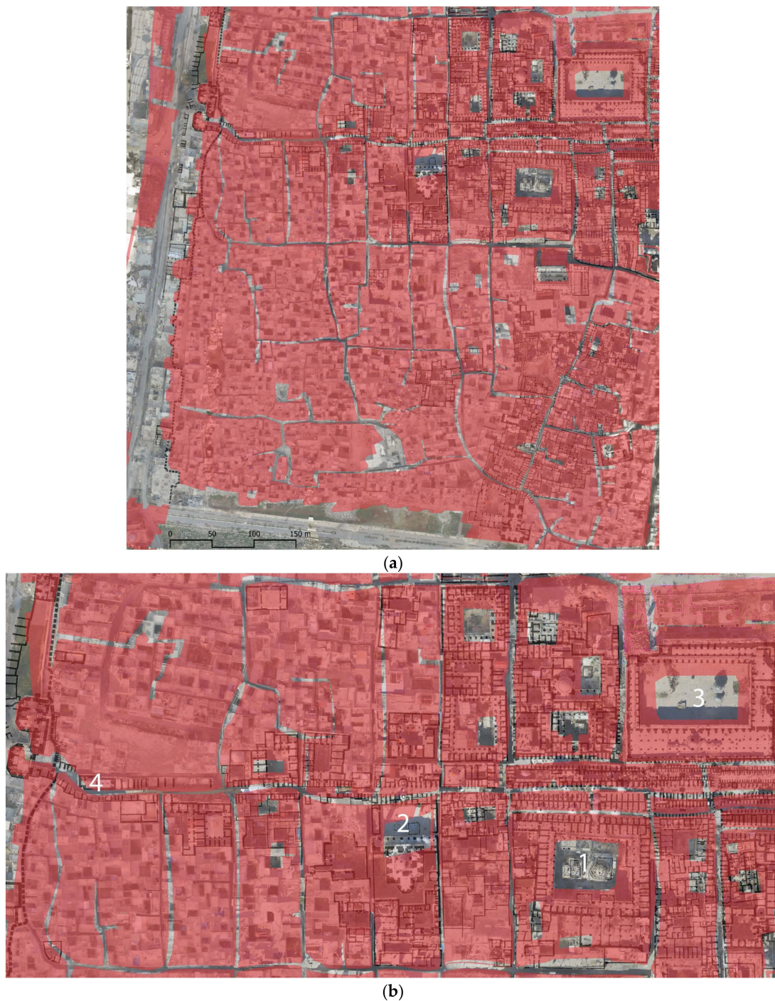
Figure 6. (a) The geo-referenced Ottoman map (in light red) and the BTU map (in black) overlaid on the orthomosaic (in RGB values) created in QGIS by the author. (b) An enlarged section of the geo-referenced Ottoman map focusing on the northern part of the studied area.
