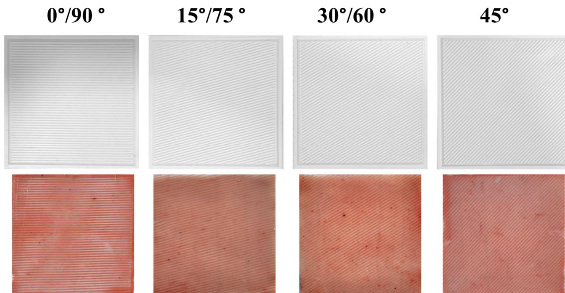
**Figure 2.** Different molds and synthetic skin with varying angles.
