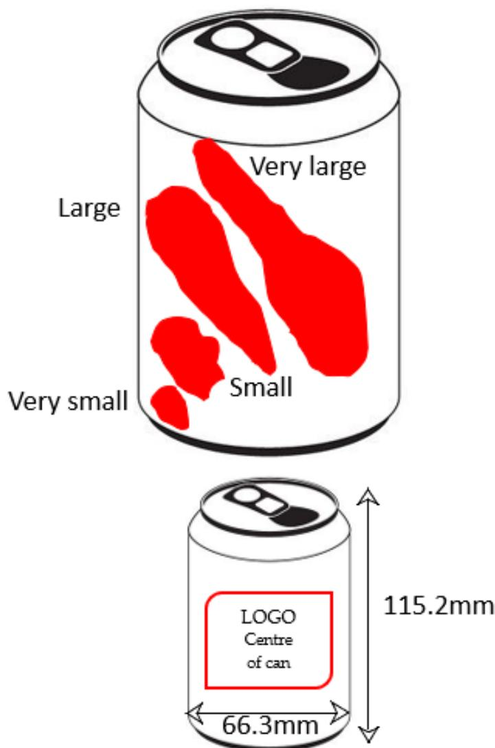
**Figure 4.** Diagrammatic representation of the categorisation of beer can perforation denoted by the red shapes increasing in size from those categorized as very small to those categorized as very large.
