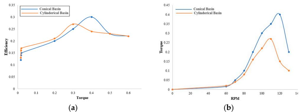
**Figure 4.** (a) Relationship between efficiency and torque of the conical and cylindrical basin. (b) Relationship between RPM and torque of conical and cylindrical basin.
