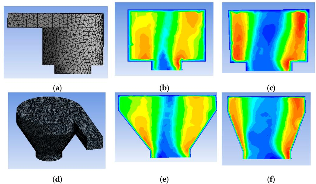
**Figure 2.** (a) Meshed cylindrical basin model; (b,c) Vortex pool of cylindrical basin; (d) Meshed conical basin model; (e,f) Vortex pool of conical basin.
