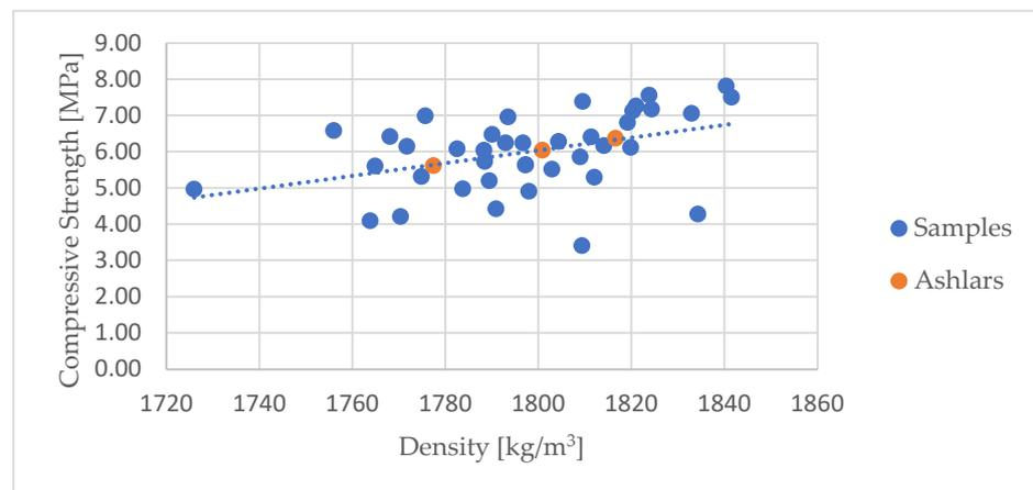
**Figure 4.** Correlation between density and compressive strength for the individual samples (blue dots) and each of the ashlars (orange dots). The linear regression is shown by a dotted blue line.
