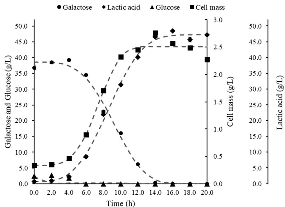
**Figure 1.** Batch fermentation kinetics of lactic acid by *Lactobacillus pentosus* from the Man-Rugosa-Sharpe medium containing initial galactose and glucose concentrations similar to *Kappaphycus alvarezii* hydrolysates. Operating conditions: pH 6, 37 °C, and 150 rpm. Standard errors in sampling were  $\leq 1$ .
