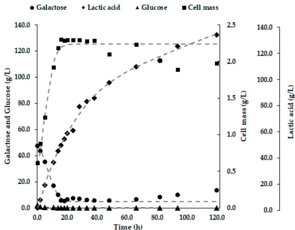
**Figure 4.** Extended continuous fed-batch fermentation kinetics of lactic acid by acclimatized *Lactobacillus pentosus* from detoxified *Kappaphycus alvarezii* hydrolysates in a 2L bioreactor with a 1L working volume. The reactor operated as a simple batch up to 14 h of fermentation, when a 400 g/L galactose solution was injected at a constant 2 mL/h flow rate. Operating conditions: pH 6, 37 °C, and 150 rpm. Standard errors in sampling were  $\leq 1$ .
