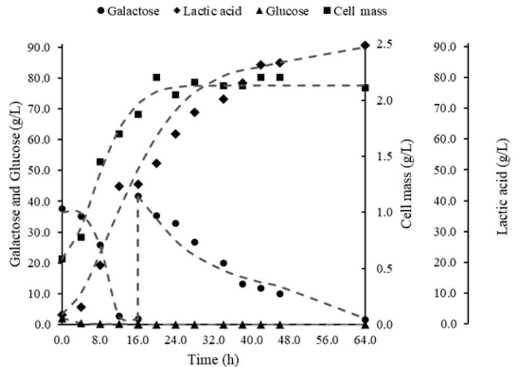
**Figure 3.** Pulse fed-batch fermentation kinetics of lactic acid by acclimatized *Lactobacillus pentosus* from detoxified *Kappaphycus alvarezii* hydrolysates in a 2L bioreactor with a 1L working volume. After initial simple batch operation, a 400 g/L galactose solution was injected at 16 h elevating concentration close to initial values. Operating conditions: pH 6, 37 °C, and 150 rpm. Standard error in sampling were  $\leq 1$ .
