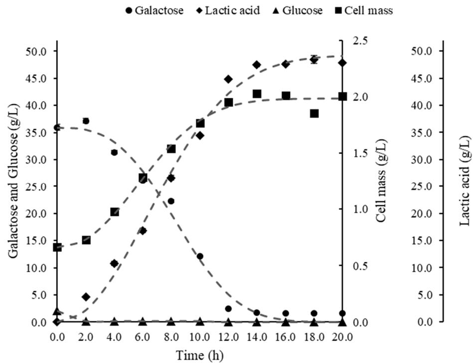
**Figure 2.** Batch fermentation kinetics of lactic acid by acclimatized *Lactobacillus pentosus* from detoxified *Kappaphycus alvarezii* hydrolysates in a 2L bioreactor with a 1L working volume. Inoculum size of 0.6 g/L. Operating conditions: pH 6, 37 °C, and 150 rpm. Standard errors in sampling were  $\leq 1$ .
