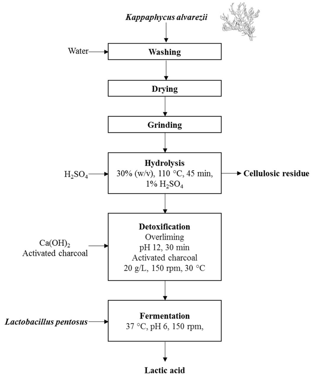
**Figure 5.** *Kappaphycus alvarezii* biorefinery scheme for lactic acid production. Filtration steps for hydrolysis and detoxification are omitted.
