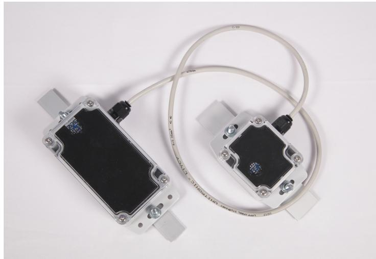
**Figure 7.** Hardware of the dual-sensor unit (with metal strips for attachment via cable ties).
