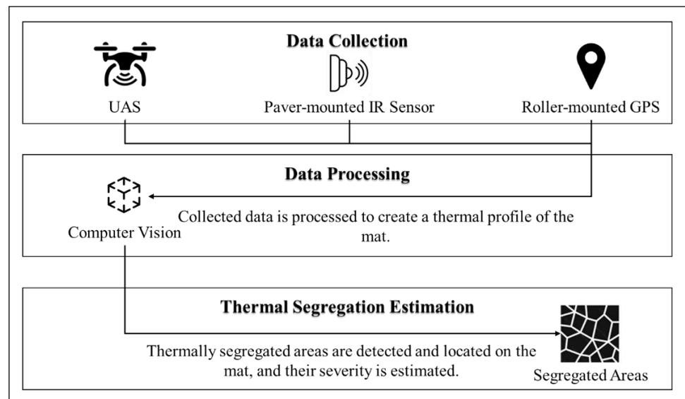
**Figure 5.** Automated HMA inspection framework.
