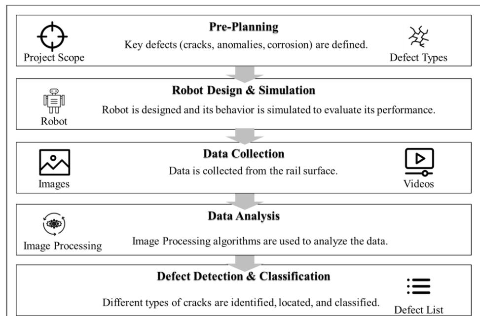
**Figure 9.** Robotic railway inspection framework.
