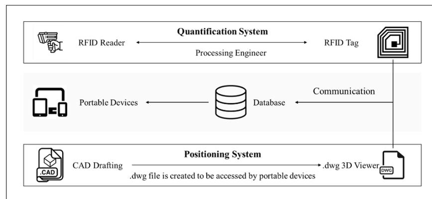
**Figure 13.** Automated falsework inspection framework [44].
