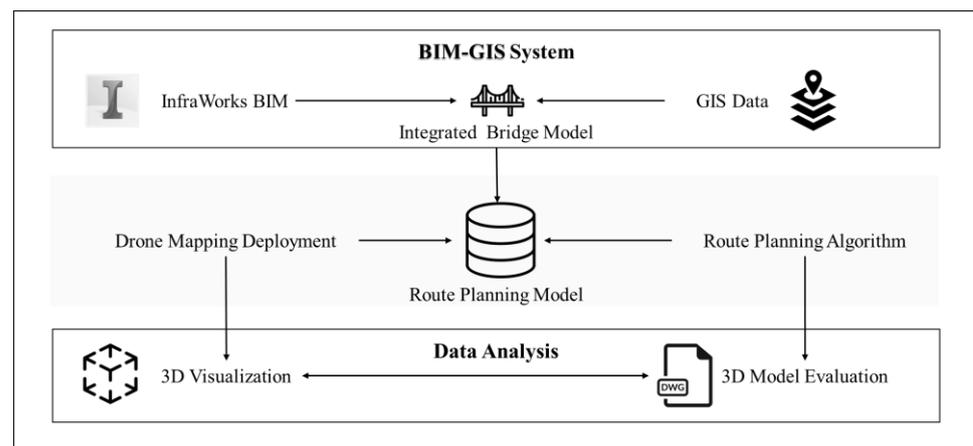
Figure 8. BIM-GIS route planning framework, proposed by [25].
