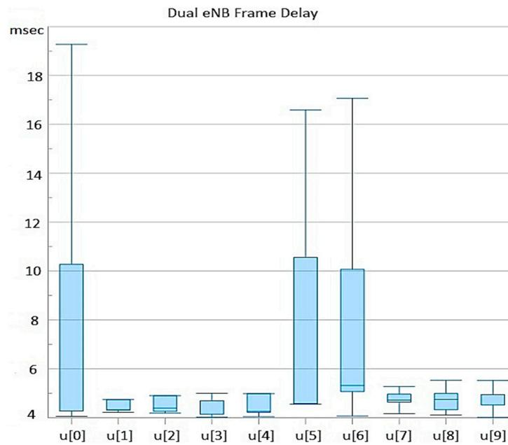
Figure 5. UEs’ simulated frame delay (dual eNB).
