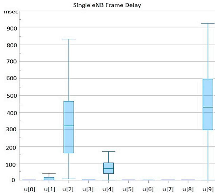
**Figure 4.** UEs’ simulated frame delay (single eNB).
