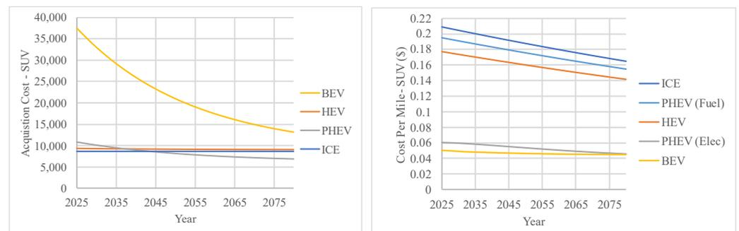
**Figure 8.** Acquisition cost (left) and cost per mile (right) for the different vehicle powertrains for the SUV in time based on advances in battery, electronics, and engine technology.
