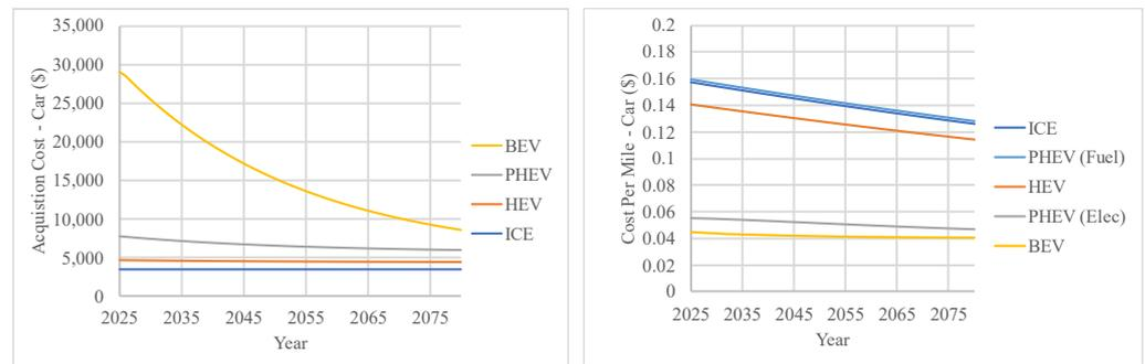
**Figure 7.** Acquisition cost (left) and cost per mile (right) for the different vehicle powertrains for the sedan in time based on advances in battery, electronics, and engine technology.
