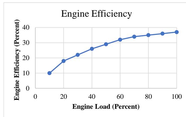
**Figure 2.** Approximation used for engine efficiency as a function of engine load based on data in [23]. Note this curve is a general curve for a modern turbocharged, direct injection engine.
