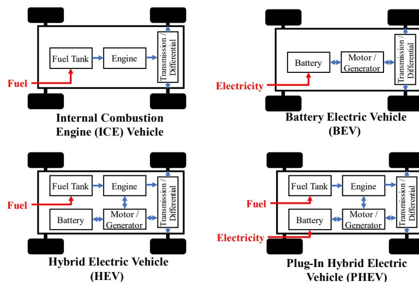
**Figure 6.** Vehicle architectures considered in this analysis.
