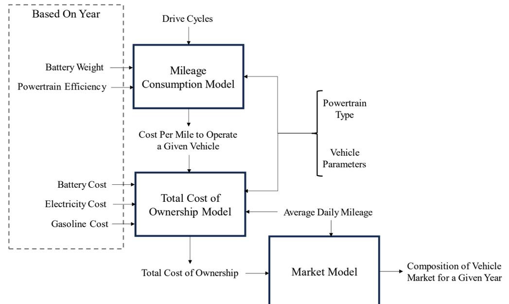
**Figure 1.** The series of models used in this study. The study used three models that calculated the cost per mile for different powertrains, the total cost of ownership for each type of vehicle, and the makeup of the market based on the overall cost of each vehicle.
