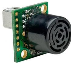
(a) Ultrasonic sensor (source: MaxBotix).
