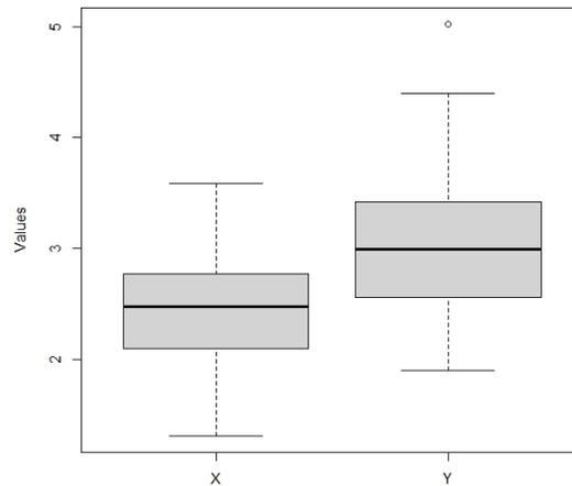
**Figure 4.** Boxplots of carbon fibre breaking strengths at gauge lengths 20 mm (left) and 10 mm (right). The circles denote outliers, hereby considered as being outside the range  $(Q_1 - 1.5(Q_3 - Q_1), Q_3 + 1.5(Q_3 - Q_1))$ , where  $Q_1$  and  $Q_3$  are the first and third quartiles of the dataset.
