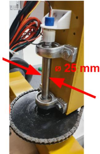
**Figure 10.** Rotation axis and the associated rotary potentiometer.
