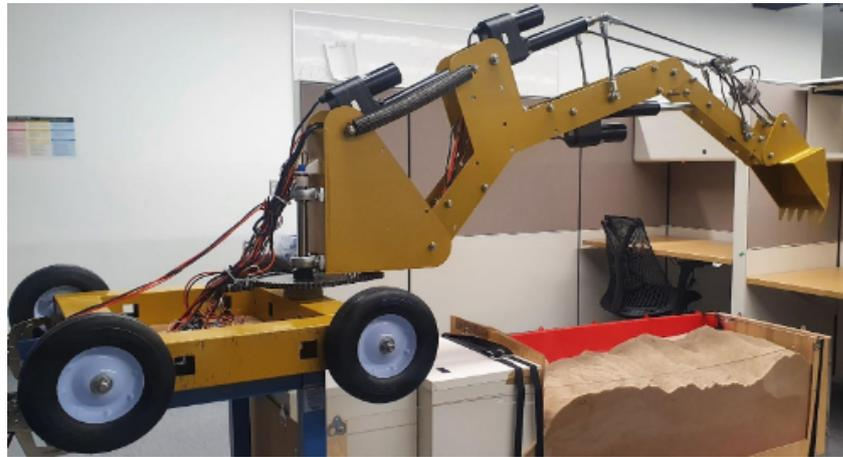
**Figure 5.** The fabricated excavator and the testbed.
