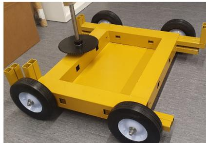
**Figure 11.** The lower structure of the excavator.
