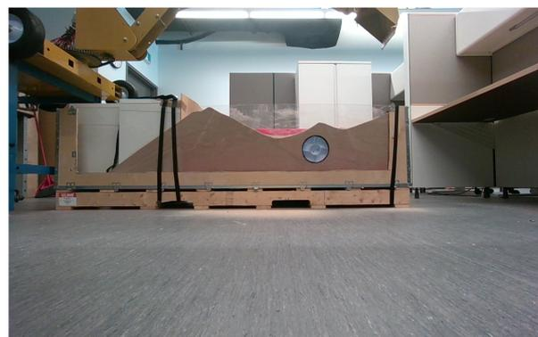
Figure 23. A pipe (white circle) was buried underground to perform the role of an underground obstacle.
