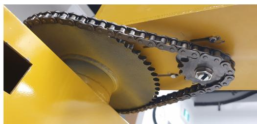
**Figure 9.** The drive chain for the swing motion.
