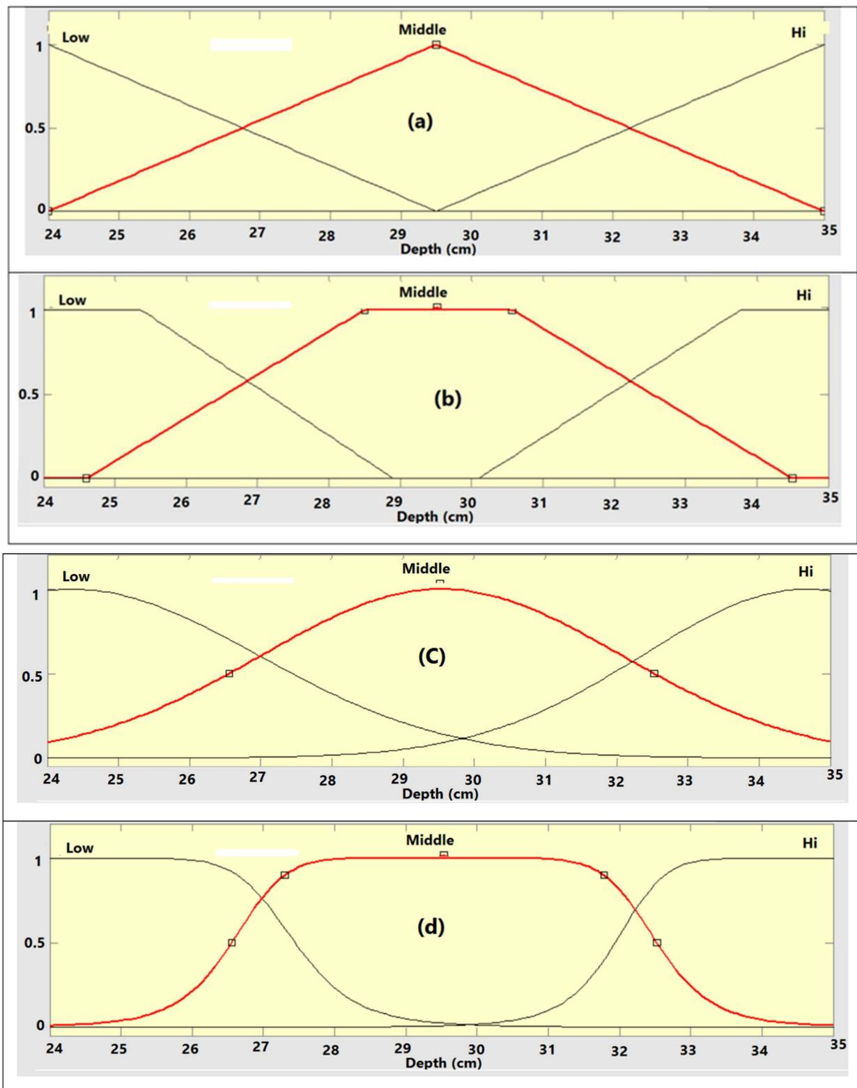
**Figure 8.** Different membership functions used for input variables (a) Triangular, (b) Trapezoidal, (c) Gaussian, (d) Bell-shaped.
