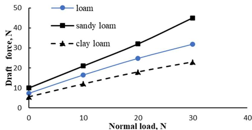
**Figure 6.** Variation of draft force versus vertical load.
