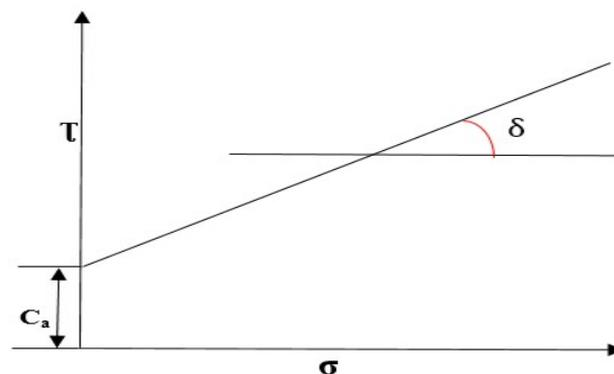
**Figure 2.** Shear stress versus normal stress to determine the soil adhesion and external friction angle.
