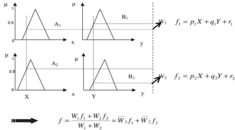
Figure 9. Schematic of fuzzy inference system: Takagi-Sugeno.
