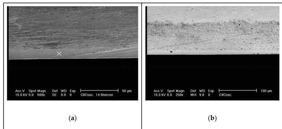
**Figure 3.** SEM image of the cross-section of the sample thickness. (a) Tantalum carbide; (b) titanium nitride.
