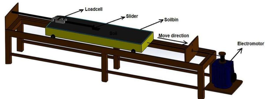
**Figure 5.** Schematic of developed device for measuring external soil friction coefficient and adhesion.
