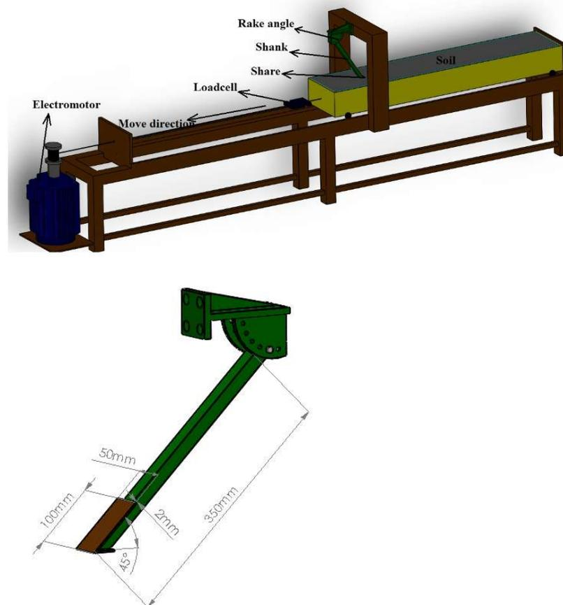
**Figure 7.** Laboratory soil bin used to perform soil cutting tests (top); geometry of coated blade on the tine (bottom).
