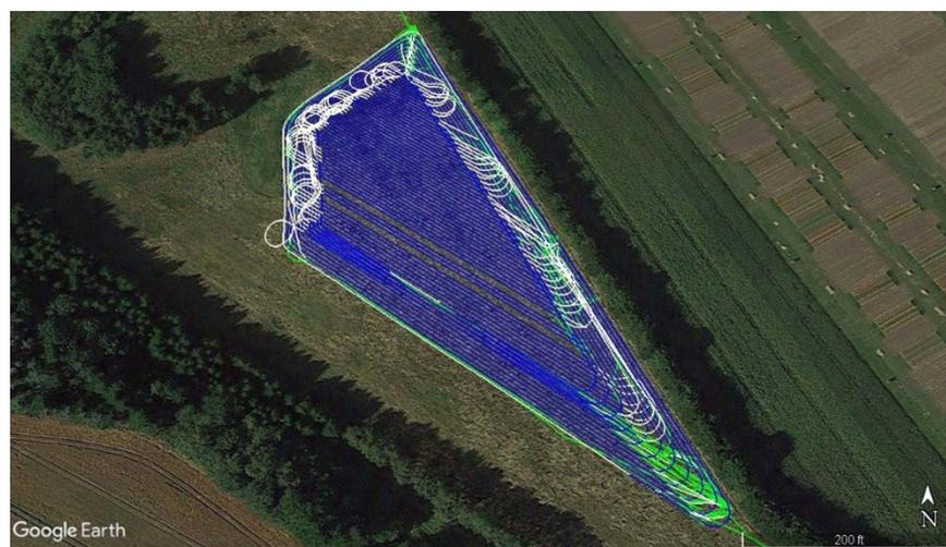
**Figure 3.** Plotted coordinates of the robot based on different task (time/distance) elements. Green color represents manual driving; blue is for automatic and working mode; and white is for automatic and nonworking mode of the robot.
