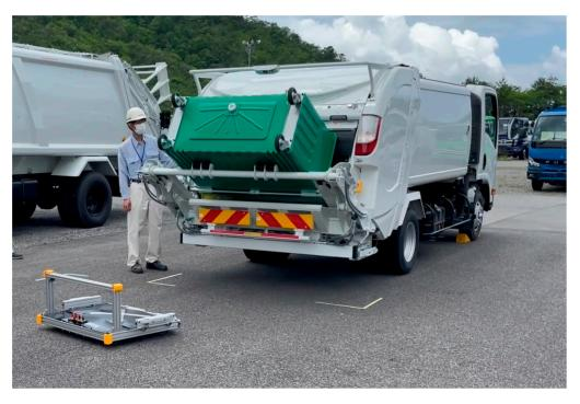
**Figure 2.** Contactless collection device that requires residents to dispose of waste in collective (green) waste containers. source: [33].
