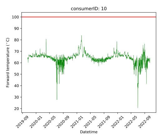
**Figure 3.** Forward temperature for a consumer with no irregular operation depicted by the green line. It displays low forward temperatures in the summer months due to no consumption in some hours leading to natural cooling of water in the system. The new threshold is depicted by the red line.
