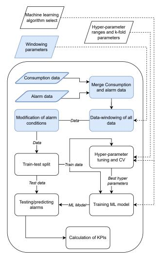
**Figure 6.** Fault prediction framework for the development phase. Blue indicates that the step was explained in the Case Study and Preprocessing Section. KPI = key performance indicator.
