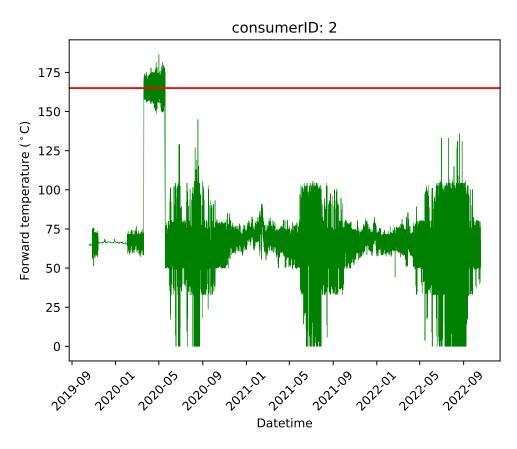
**Figure 1.** Forward temperature for one of the 5 consumers using the original fault definition. Here, it can be seen how long the first fault persists. The triggering threshold for alarm 8 is 165 °C, depicted by the horizontal red line.
