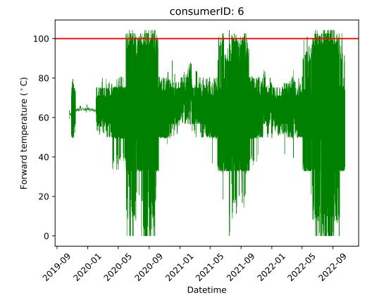
**Figure 2.** Forward temperature depicted by the green line with both extremely fluctuating forward temperature (which can be acceptable, as the water cools in the heating system if no heat is used, seen especially in the summer months) and violations of the new threshold depicted by the red line.
