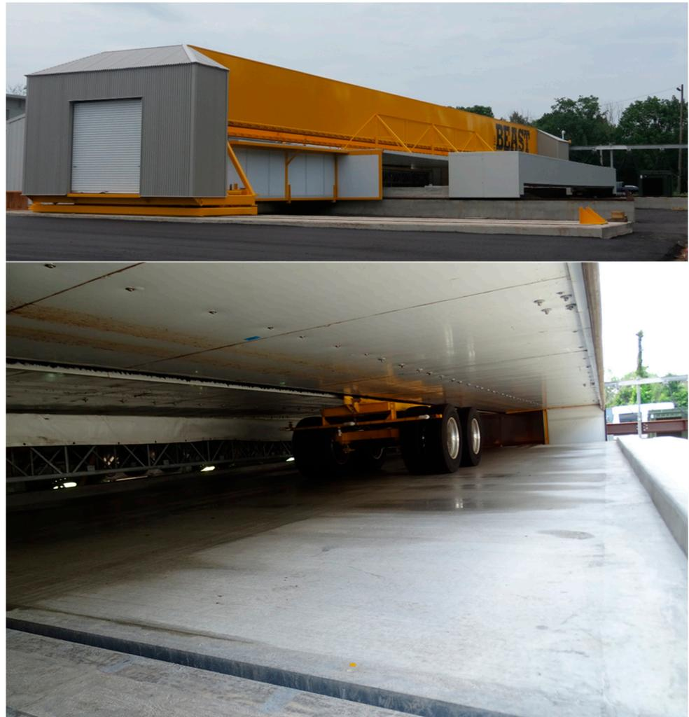
**Figure 15.** The loading device that represents the truck axel loads at the BEAST<sup>®</sup> facility.
