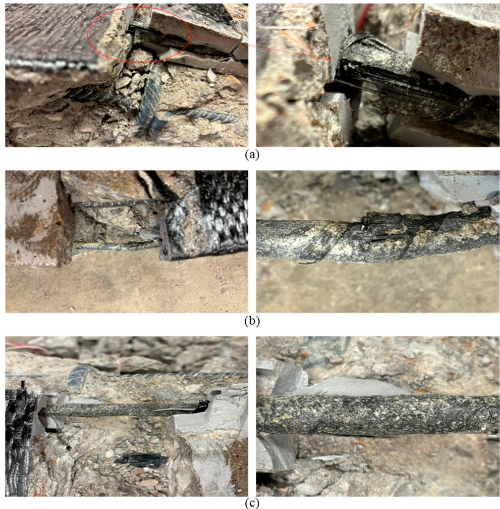
**Figure 16.** Various failure modes of RC beams strengthened with NSM-CFRP, (a) type NU beams, failed by the CFRP bar rupture, (b) type NSU beams, failed by the CFRP bar rupture, (c) type NSU beams, failed by sudden spilling of the epoxy cover.
