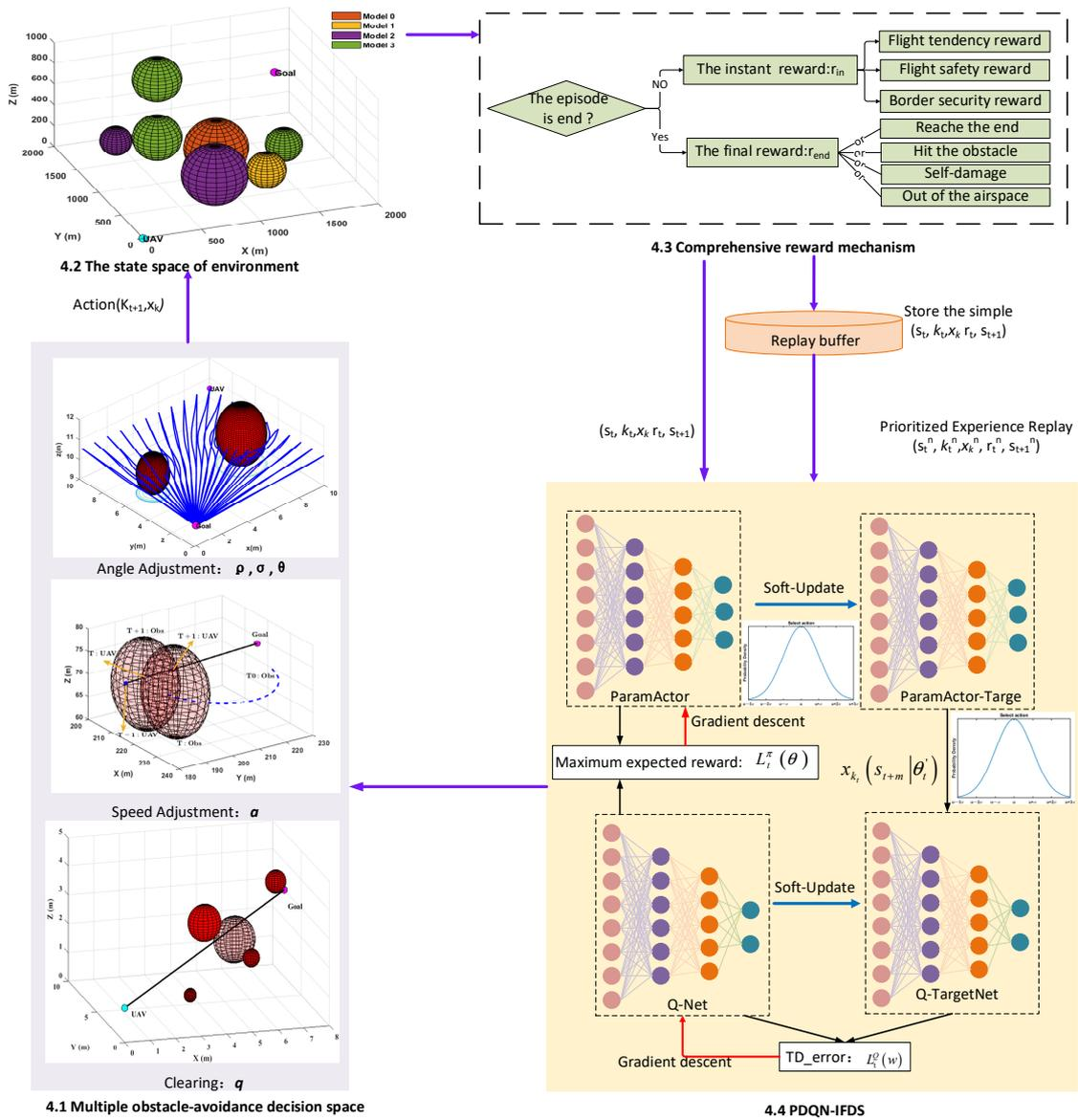
Figure 6. Flow chart of the autonomous path planning algorithm of drones based on MSAO2H.
