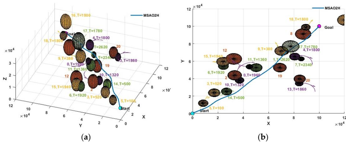
Figure 14. Result of path planning based on MSAO2H in a complex environment: (a) three-dimensional path and (b) X-Y plane projection.
