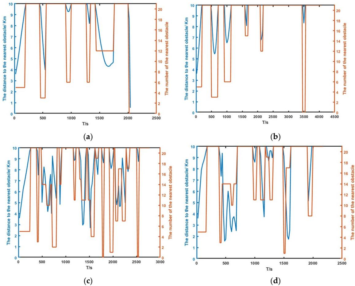
**Figure 15.** Distance to the nearest obstacle during flight; (a) based on the DDPG; (b) based on the DDPG-IFDS; (c) based on the PDQN; (d) based on MSAO2H.
