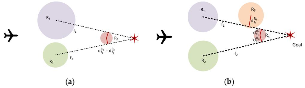
**Figure 5.** Benefits of obstacle clearance: (a) the influence of obstacle radius and (b) the influence of obstacles distribution.
