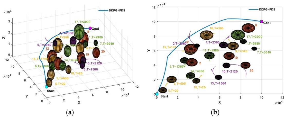
Figure 12. Result of path planning based on the DDPG-IFDS in a complex environment: (a) three-dimensional path and (b) X-Y plane projection.
