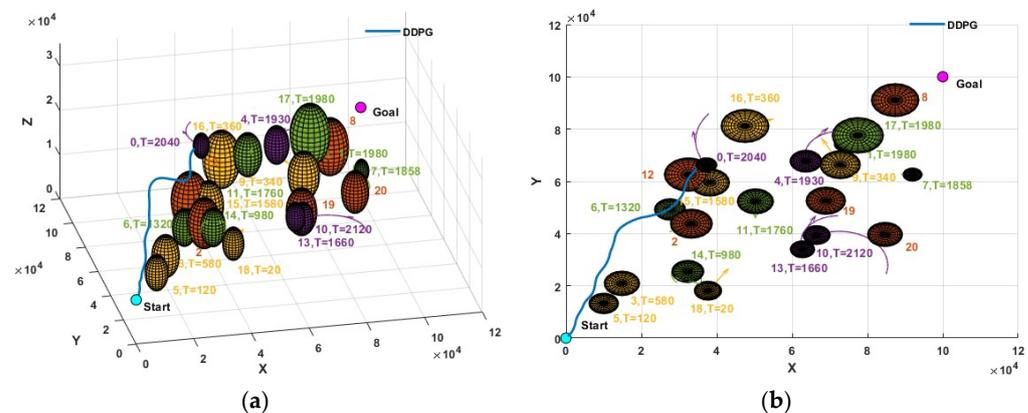
**Figure 11.** Result of path planning based on the DDPG in a complex environment: (a) three-dimensional path and (b) X-Y plane projection.
