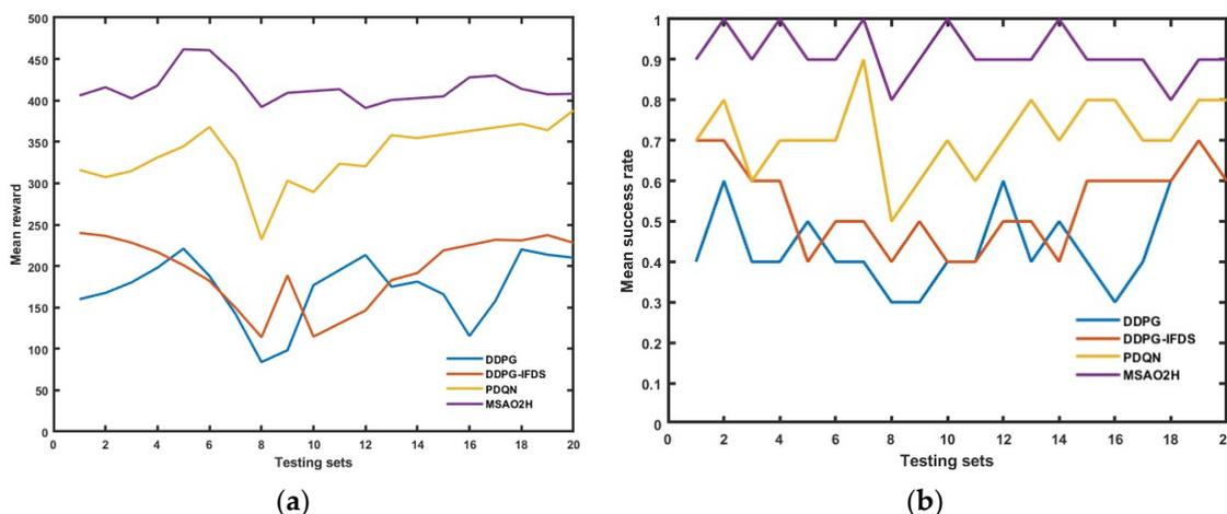
**Figure 16.** Test results of path planning in random obstacle environments: (a) the average reward and (b) the average success rate.
