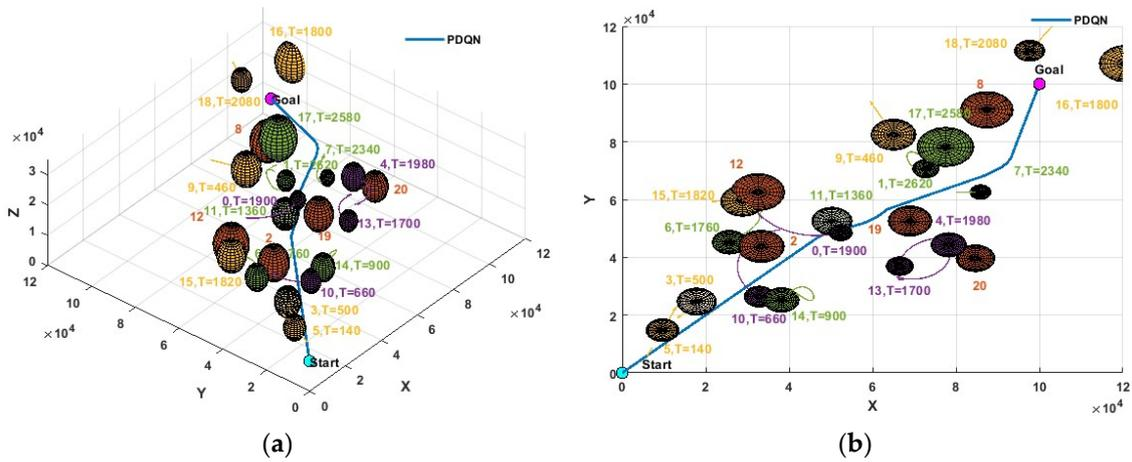
Figure 13. Result of path planning based on the PDQN in a complex environment: (a) three-dimensional path and (b) X-Y plane projection.
