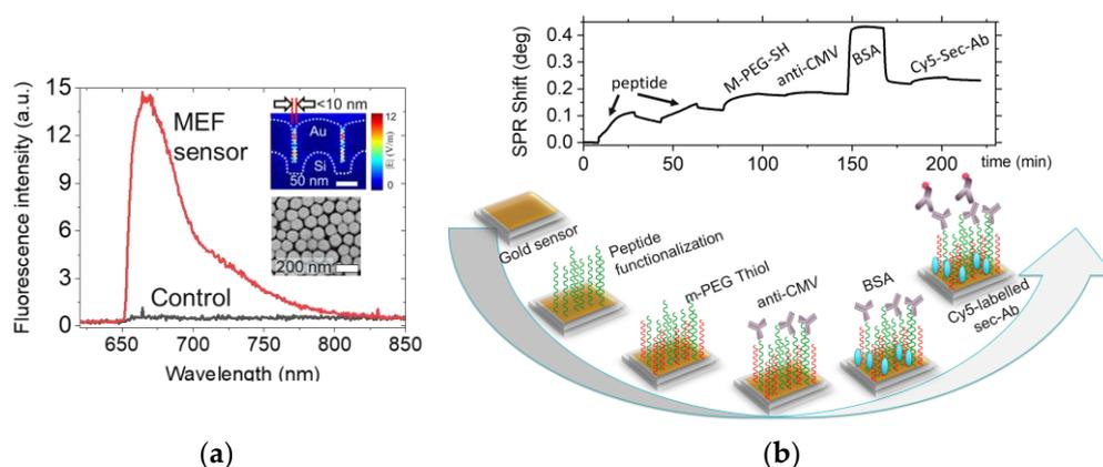
**Figure 1.** Plasmonic detection of peptide–protein interactions (a) Gold nanoarrays (SEM-top view), and numerically simulated electromagnetic field profiles showing sub-10 nm electromagnetic hotspots; plot compares fluorescence intensities on MEF sensors and on control surface (equivalent to the gold SPR chips used in (b)) (b) Illustration of the assay steps and the corresponding experimentally measured SPR shifts.
