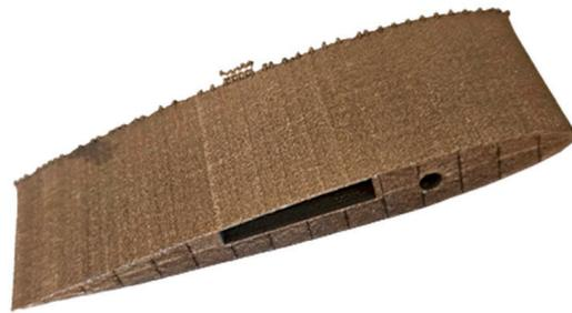
Figure 2. Model 2—metal 3D-printed airfoil.
