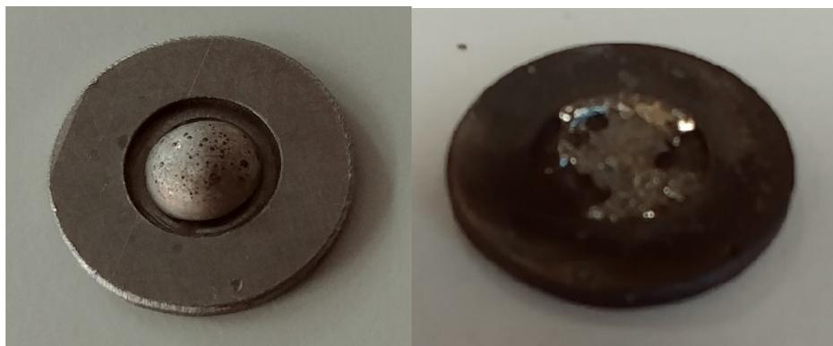
**Figure 5.** **Left:** Niobium disc with  $[^{76}\text{Se}]\text{CoSe}$  nugget on top. **Right:** Niobium disc with hot-pressed  $[^{76}\text{Se}]\text{CoSe}$ .
