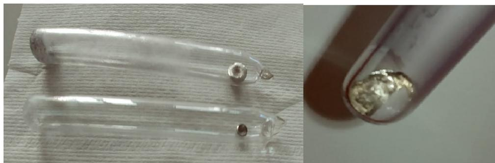
**Figure 4.** Evacuated quartz glass ampules containing CoSe after heating in the furnace at 1200 °C for 60 min. **Left:** Closed ampule—loose metallic glassy nuggets with no remains. **Right:** CoSe with metallic shine—easily removeable from quartz glass.
