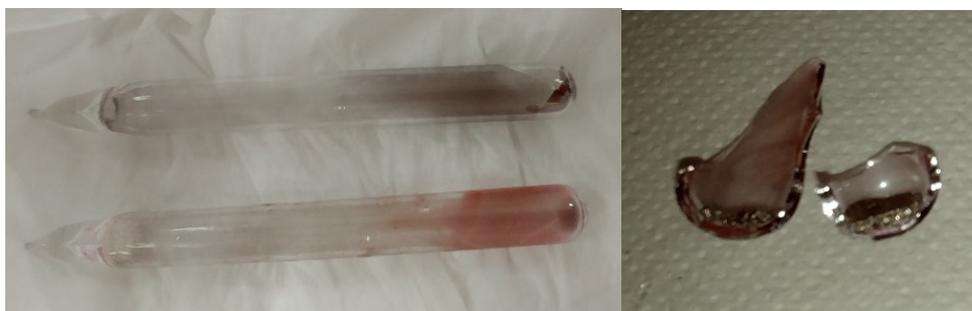
**Figure 3.** Evacuated quartz glass ampoules containing CoSe after heating in the furnace at 1200 °C for 60 min. **Left:** Closed ampule—silvery shining amorphous deposits together with grayish or reddish remains at the inner surface of the quartz glass ampule. **Right:** opened ampule—porous and brittle CoSe is strongly sticking to the quartz surface.
