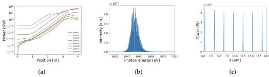
**Figure 8.** Three-dimensional simulation results of UC-XRAFEL with 3  $\mu$ m modulated electron beams. Each plot shows (a) the gain curve (b) the output spectrum, and (c) the power profile. A maximum power of 44 GW is reached after the sixth pass.
