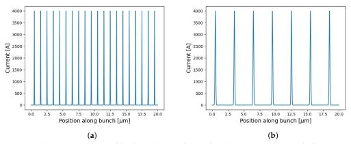
**Figure 2.** (a) 1  $\mu$ m current profile along the bunch length. The beam is composed of 20 Gaussian functions, each separated by 1  $\mu$ m. (b) 3  $\mu$ m current profile along the bunch length, with separation 3  $\mu$ m.
