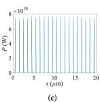
**Figure 3.** 1D UC-XRAFEL simulation results for the 1-μm current modulation. (**a**) The gain curves after each recirculation pass for optimal tapering [37]. (**b**) The output spectrum after the 5th pass. (**c**) The power profile of the out-coupled radiation for the 5th pass, with a maximum power along the bunch peaking at 80 GW.
