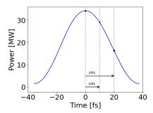
**Figure 7.** Seed profile for the 7th pass of the 1  $\mu$ m current profile. A 10–20 fs offset of the seed input from the electron bunch length results in a partial decrease of the input seed power.
