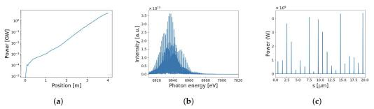
**Figure 6.** Three-dimensional simulation results of a single-pass, non-tapered SASE with 1  $\mu$ m modulated electron beams. Each plot describes (a) the gain curve, (b) the output spectrum, and (c) the power profile. The maximum output power attainable by single-pass SASE for a 1  $\mu$ m current profile is 4.5 GW.
