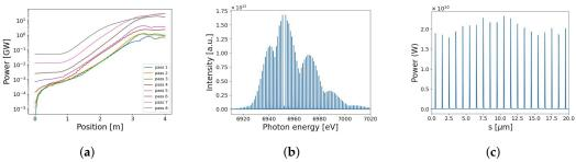
Figure 5. Three-dimensional simulation results of UC-XRAFEL with 1  $\mu$ m modulated electron beams. Each plot describes (a) the gain curves after each pass through the cavity, (b) the output spectrum after the 7th pass, and (c) the power profile of the out-coupled radiation for the 7th pass. The maximum output power along the bunch peaks at 25 GW.
