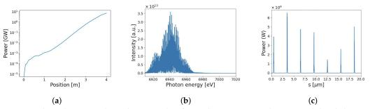
**Figure 9.** Three-dimensional simulation results of a single-pass SASE with 3  $\mu$ m modulated electron beams. (a) Gain curve, (b) output spectrum, and (c) power profile for SASE with no tapering. The maximum power along the bunch peaks at 6.5 GW.
