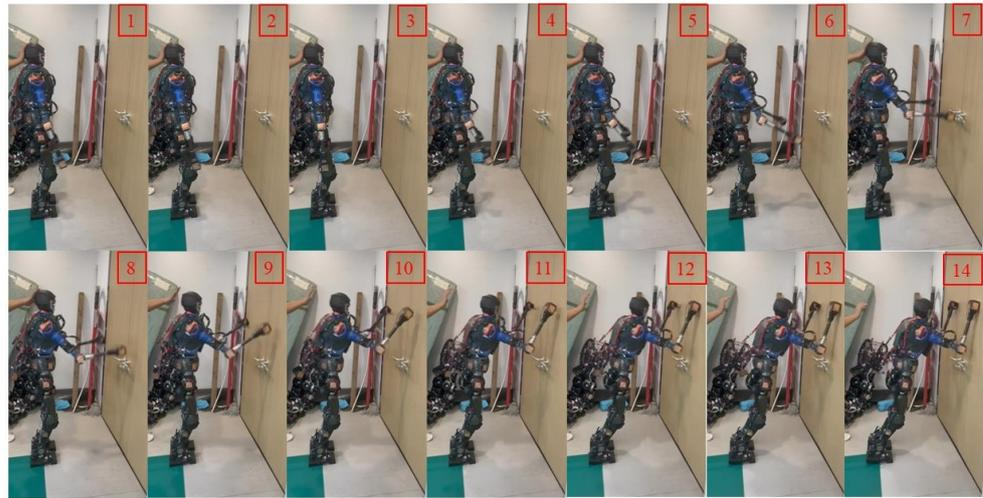
**Figure 16.** Experiment on the robot’s actual fall and wall support.
