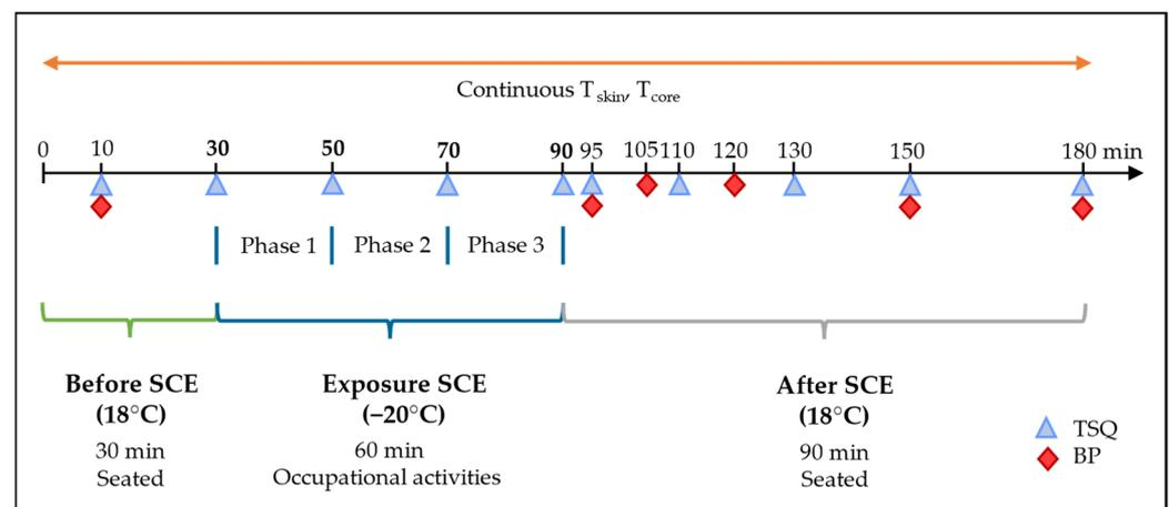
**Figure 1.** Testing schedule for each participant before, during, and after severe cold exposure.
