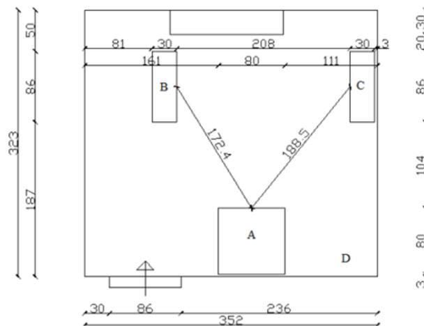
**Figure 2.** The climatic chamber ground plan with dimensions in centimetres.
