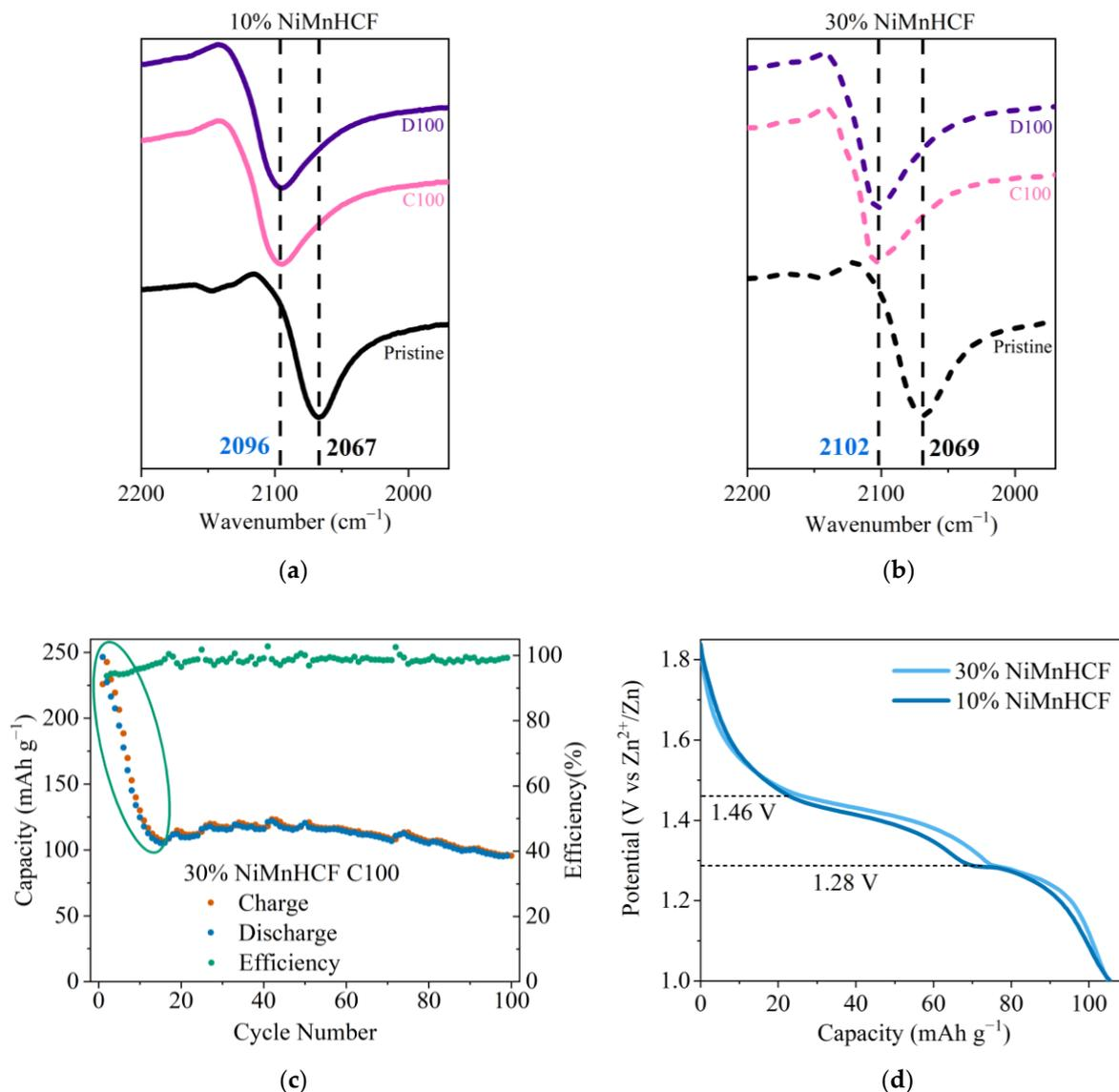
**Figure 6.** ATR-FT-IR analysis results of pristine and cycled electrodes of (a) 10%NiMnHCF, (b) 30%NiMnHCF; GCPL data of (c) stability and efficiency of the C100 of 30%NiMnHCF, (d) discharge curve after the stabilization of 10% and 30%NiMnHCF (extracted from same cycle).
