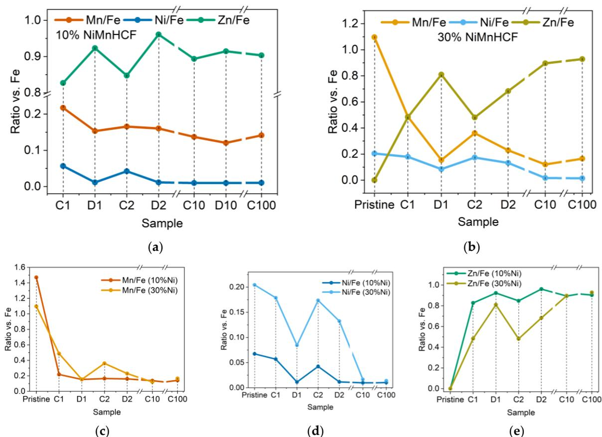
**Figure 3.** 2D-XRF semi-quantitative analysis results showing the dynamics of Mn, Ni, and Zn vs. Fe in ex situ electrodes for the (a) 10%NiMnHCF series and the (b) 30%NiMnHCF series. The dynamics of (c) Mn vs. Fe, (d) Ni vs. Fe, and (e) Zn vs. Fe in the NiMnHCF electrodes.
