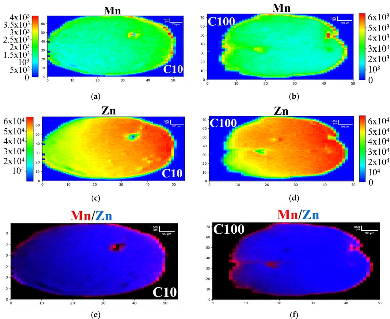
**Figure 5.** Normalized 2D-XRF maps of 30%NiMnHCF ex situ electrode: (a) Mn C10, (b) Mn C100, (c) Zn C10, (d) Zn C100. Intensity scale is color-based (red = high intensity; blue = low intensity). (e) Mn and Zn overlay of C10, (f) Mn and Zn overlay of C100 (Mn in red, Zn in blue). Length scale: Vertical bar  $1000 \mu\text{m}$  ( $200 \mu\text{m} \times 5 \text{ px}$ ), horizontal bar  $700 \mu\text{m}$  ( $140 \mu\text{m} \times 5 \text{ px}$ ).
