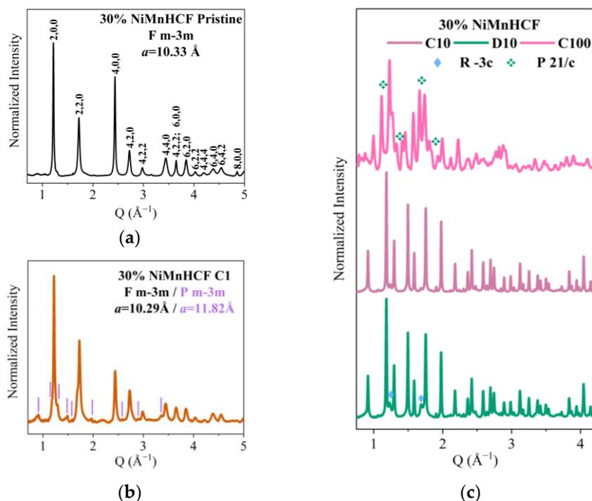
**Figure 7.** PXRD measurement results of 30%NiMnHCF ex situ electrodes: (a) Pristine, (b) C1, (c) C10, D10, and C100.
