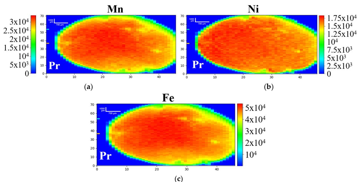
**Figure 1.** Normalized 2D-XRF maps of 30%NiMnHCF pristine ex situ electrode: (a) Mn, (b) Ni, (c) Fe. Intensity scale is color-based (red = high intensity; blue = low intensity). Length scale: Vertical bar 1000  $\mu\text{m}$  (200  $\mu\text{m} \times 5$  px), horizontal bar 700  $\mu\text{m}$  (140  $\mu\text{m} \times 5$  px).
