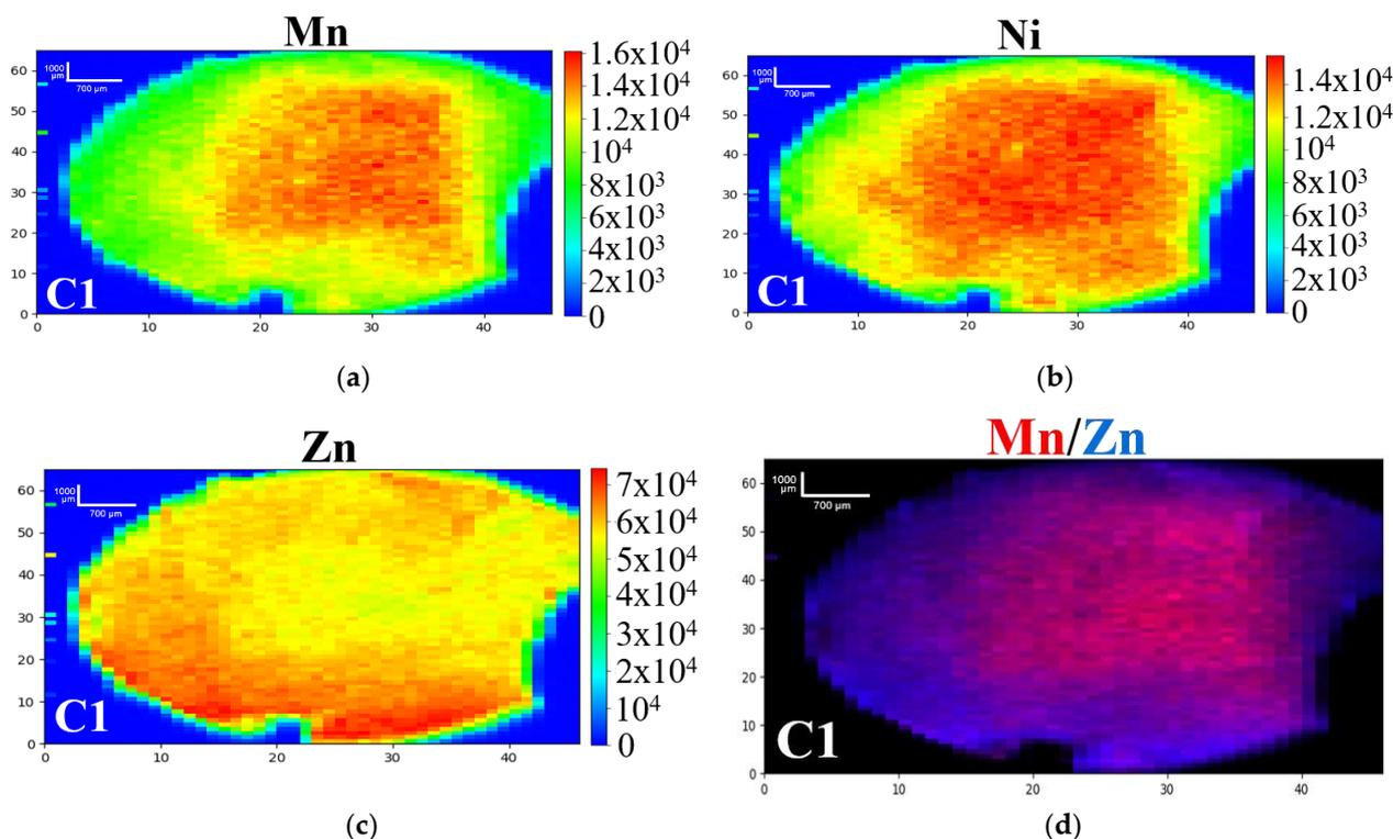
**Figure 2.** Normalized 2D-XRF maps of 30%NiMnHCF C1 ex situ electrode: (a) Mn, (b) Zn, (c) Ni, (d) Mn and Zn overlay (Mn in red, Zn in blue). For (a–c), intensity scale is color-based (red = high intensity; blue = low intensity). Length scale: Vertical bar 1000  $\mu\text{m}$  (200  $\mu\text{m} \times 5$  px), horizontal bar 700  $\mu\text{m}$  (140  $\mu\text{m} \times 5$  px).
