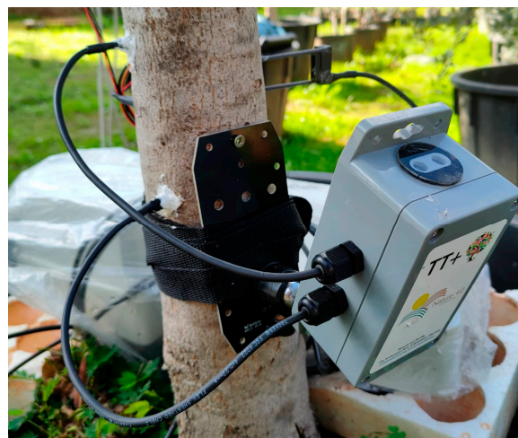
Figure 3. TreeTalker ® mounted on an olive trunk.
