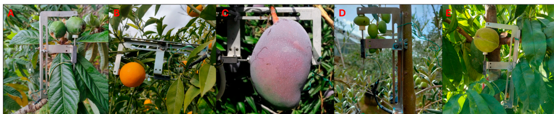
Figure 4. LVDT fruit gauges mounted in loquat (A), orange (B), mango (C), olive (D), and peach (E) fruit.
