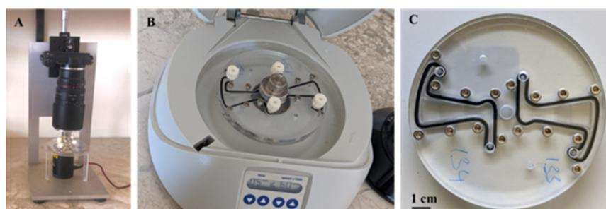
**Figure 2.** SIMPAQ setup. (A) SIMPAQ microscope with the disc ready for examination; (B) centrifuge; and (C) the lab-on-a-disc (LoD).
