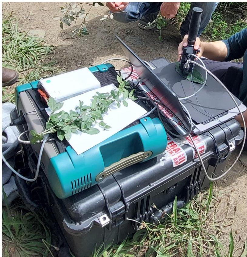
**Figure 2.** Reflectance data collection over a leaf, during fieldwork, with a spectroradiometer ASD FieldSpec® 4.
