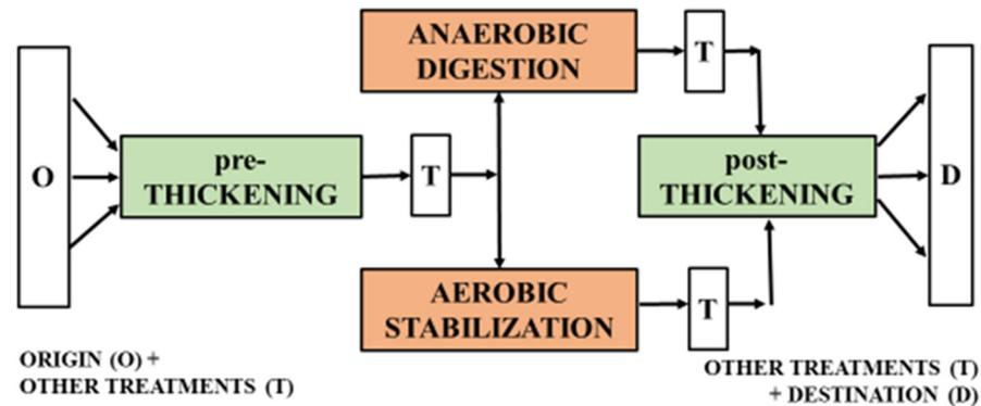
**Figure 2.** Technical “*Hubs*” in sludge processing from origin to destination.
