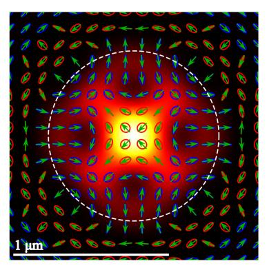
**Figure 2.** Intensity pattern at the focus for the original field (1) at n = 0, m = -2 forms a colored (yellow-red) square; green arrows mark the major axis vector of polarization ellipses: red ellipses mark a positive on-axis projection and blue ones mark a negative one. The white horizontal line is 1 um long. The white dashed circle is where a two-sided half-twisted ribbon with four half-twists and index -2 is generated.
