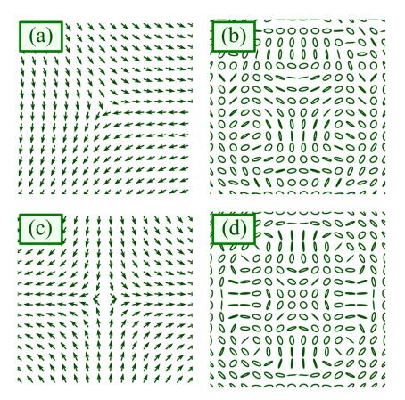
**Figure 5.** Distributions of linear polarization vectors in the initial plane of the beam (4) (**a**) and of the beam (15) (**c**), as well as distributions of the polarization ellipses in the focus plane of the beam (4) (**b**) and of the beam (15) (**d**). The numerical aperture is 0.95. The frame size is 1  $\mu$ m (**b**,**d**).
