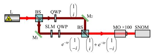
**Figure 3.** Optical setup for generating and focusing a Poincaré beam (4): L—laser with the wavelength of 532 nm; BS—nonpolarizing beam splitters; QWP—quarter-wave plate;  $M_1$  and  $M_2$ —rotatable mirrors; SLM—transmissive liquid-crystal spatial light modulator; MO—microobjective with a  $100 \times 200$  zoom (NA = 0.95); and SNOM—scanning near-field optical microscope. Red arrows show the direction of light propagation.
