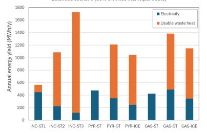
**Figure 6.** Analysis of annual energy yield in terms of electricity and usable waste heat from mixed municipal waste using nine different thermochemical processes. Data are shown for the balanced scenario.
