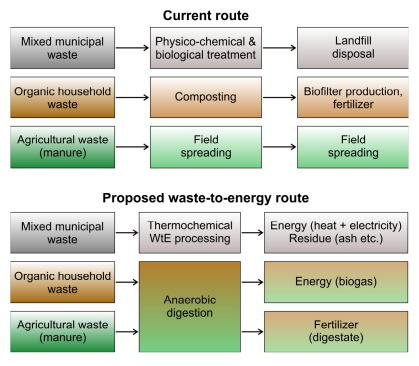
Figure 5. Current and proposed waste management of relevant waste flows in the Kočevje municipality.
