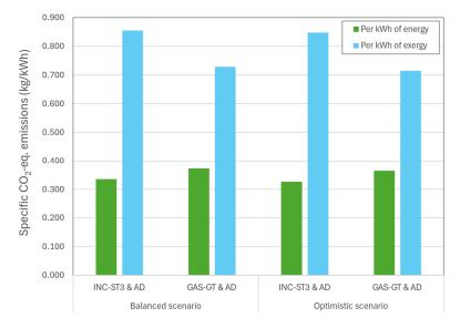
**Figure 14.** Specific CO<sub>2</sub>-eq. emissions per kWh of generated energy (electricity and heat) and exergy for different technologies and scenarios.
