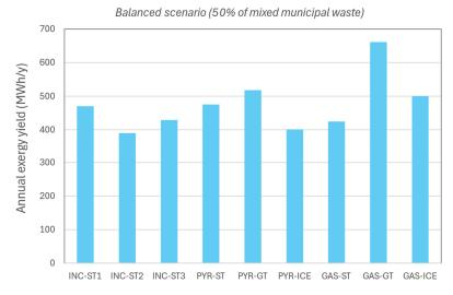
**Figure 7.** Analysis of annual exergy production using nine different thermochemical processes. Data are shown for the balanced scenario.
