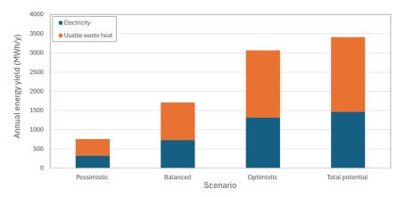
**Figure 8.** Analysis of annual energy yield in terms of electricity and usable waste heat from biodegradable municipal waste and livestock manure using anaerobic digestion and combustion of the biogas in an internal combustion engine.
