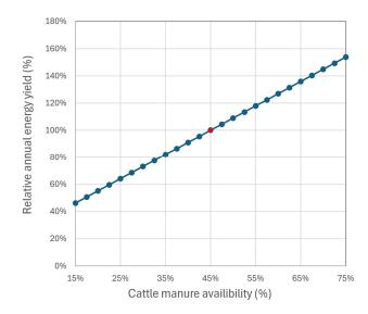
**Figure 9.** Sensitivity of the annual energy yield of anaerobic digestion towards the availability of cattle manure. The values are given relative to the base scenario using an availability of 45% (denoted with red color).
