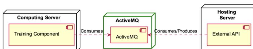
Figure 9. ActiveMQ deployment diagram.
