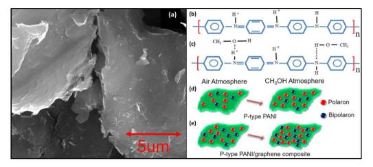
**Figure 13.** (a) FESEM images of PANI/graphene composite; (b) PANI chain; (c) hydrogen bond formation between PANI and methanol molecules; (d,e) PANI and PANI/graphene composite under methanol environment from air environment (Reprinted/adapted from [111]).
