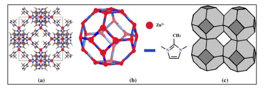
**Figure 6.** (a) ZIF-8 sodalite cage in which Zn, C, N, and H are shown in red, brown, blue, and grey, respectively; (b) ZIF-8 ball-and-stick model; (c) sodalite topology (Reprinted/adapted from [46]).
