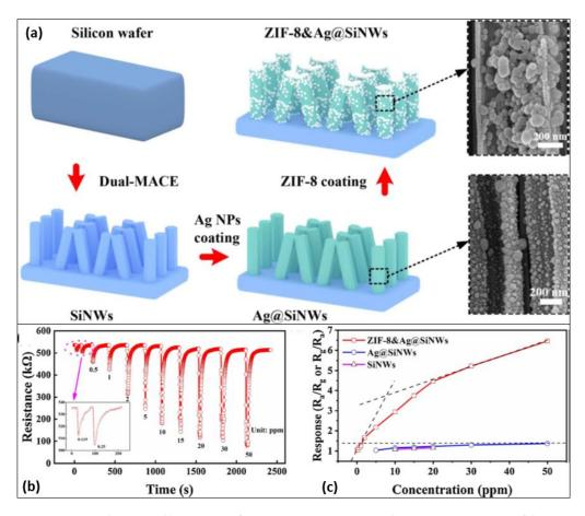
**Figure 7.** (a) Schematic illustration of SiNWs, Ag@SiNWs, and ZIF-8& Ag@SiNWs fabrication; (b) Sensor responses of ZIF-8& Ag@SiNWs upon exposure to different ethanol concentrations; (c) Response comparison to ethanol for SiNWs, Ag@SiNWs, and ZIF-8& Ag@SiNWs (Reprinted/ adapted from [49]).
