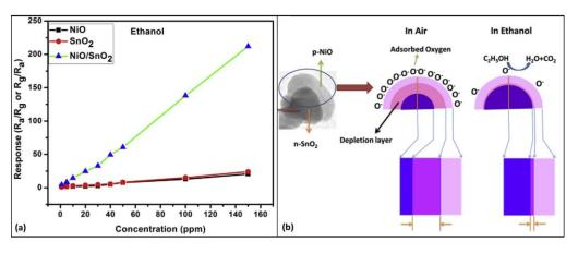
**Figure 3.** (a) Responses of NiO/SnO<sub>2</sub>, SnO<sub>2</sub>, and NiO sensors upon ethanol exposure at different concentrations at room temperature. (b) Schematic illustration of NiO/SnO<sub>2</sub> gas-sensor mechanism. (Reprinted/adapted from [31]).
