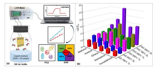
**Figure 8.** (a) Schematic illustration of the impedimetric setups for volatile organic compounds (VOCs) detection; (b) Sensor responses from each sensor in the array toward the target VOC at 80 ppm (Reprinted/adapted from [66]).
