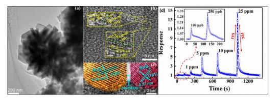
**Figure 10.** (a) TEM image of SnS/SnS<sub>2</sub> sheet; (b,c) HRTEM images of SnS/SnS<sub>2</sub> sheet; (d) Sensor responses to different methanol concentrations at room temperature (Reprinted/adapted from [83]).
