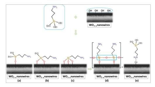
**Figure 5.** Schematic illustration of the  $WO_{3-x}$  surface silanization via oxygen bonding from the (**a**) one, (**b**) two, and (**c**) three ethoxy groups; (**d**) the polymerization of the APTES adsorbed through all three ethoxy groups; (**e**) the interaction with amino group. (Reprinted/adapted from [43]).
