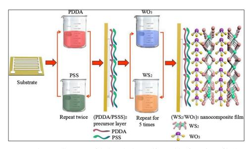
**Figure 9.** Schematic illustration of the layer-by-layer self-assembly of WS<sub>2</sub>/WO<sub>3</sub> film (Reprinted/ adapted from [75]).
