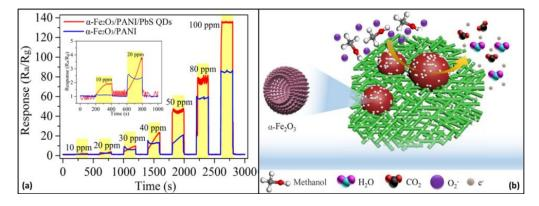
**Figure 14.** (a) Sensor responses to methanol at room temperature; (b) Schematic illustration of  $\alpha$ -Fe<sub>2</sub>O<sub>3</sub>/PANI/PbS gas sensor mechanism (Reprinted/adapted from [119]).
