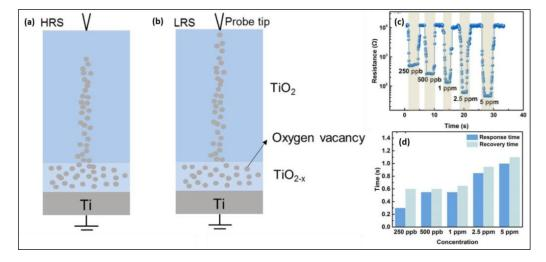
**Figure 15.** Schematic illustration of the SnS/TiO<sub>2</sub>-based gasistor in (**a**) HRS and (**b**) LRS. (**c**) Response to different methanol concentrations in HRS. (**d**) Response and recovery time to different methanol concentrations. (Reprinted/adapted from [127]).
