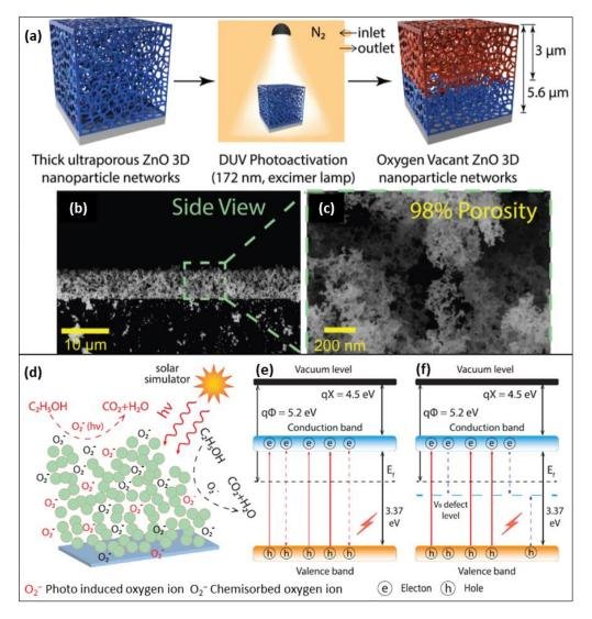
**Figure 4.** (a) Schematic illustration of DUV photoactivation for thin ultraporous ZnO nanostructure; (b,c) Cross-sectional SEM images of ZnO ultraporous nanostructure at different magnifications; (d) Schematic illustration of ethanol-sensing mechanism involving chemisorbed oxygen ions under solar irradiation; (e) Energy-band structure of pristine ZnO; (f) Energy-band structure of oxygen vacant ZnO (Reprinted/adapted from [42]).
