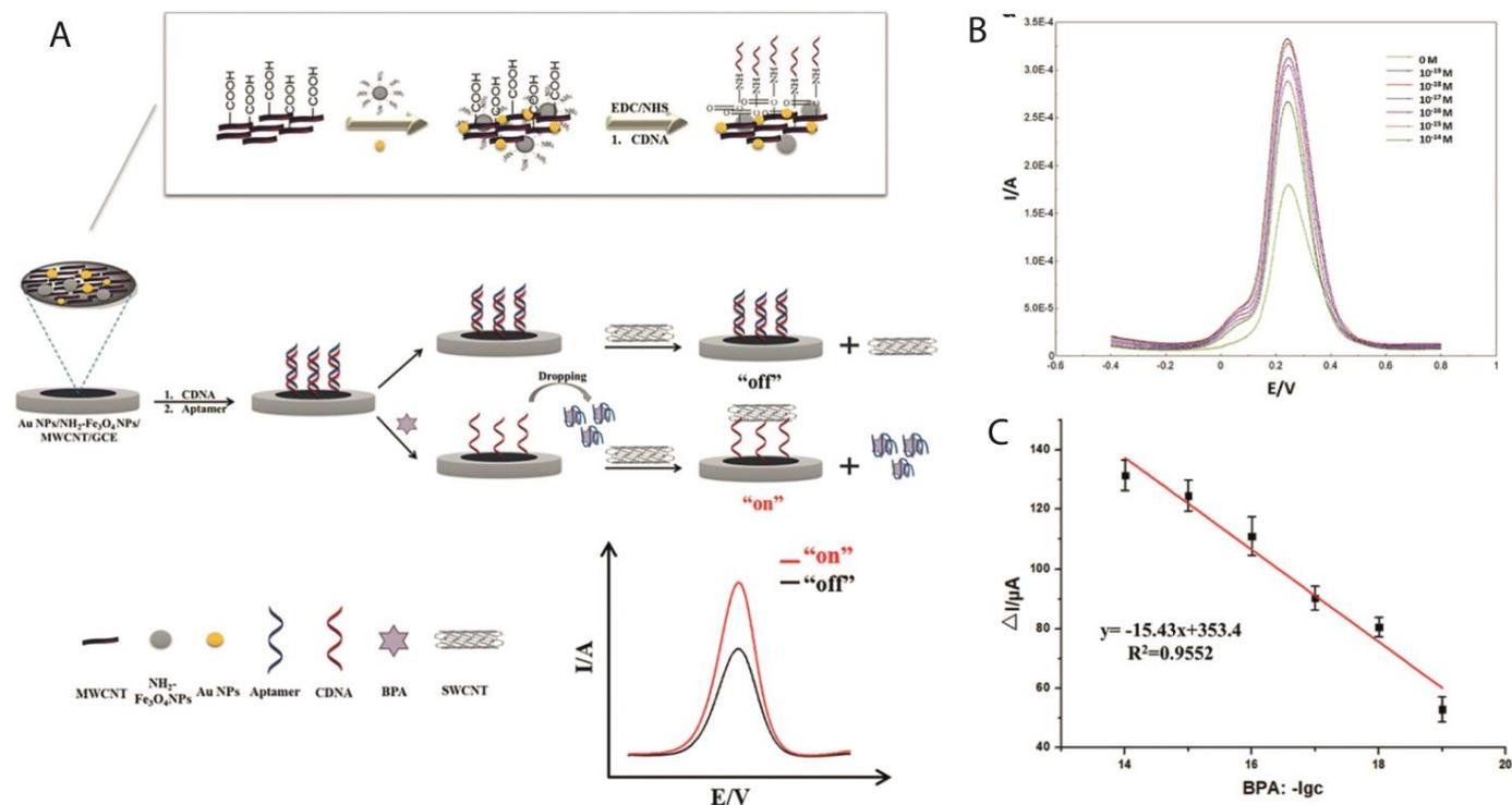
**Figure 7.** (A) Schematic diagram of the fabrication of a “signal-on” sensing model. (B) Differential pulse voltammetry responses at different concentrations of BPA ( $10^{-19}$  M,  $10^{-18}$  M,  $10^{-17}$  M,  $10^{-16}$  M,  $10^{-15}$  M,  $10^{-14}$  M) in lake water. (C) BPA calibration curve in lake water. Reprinted from reference [98] with permission from Springer Nature.
