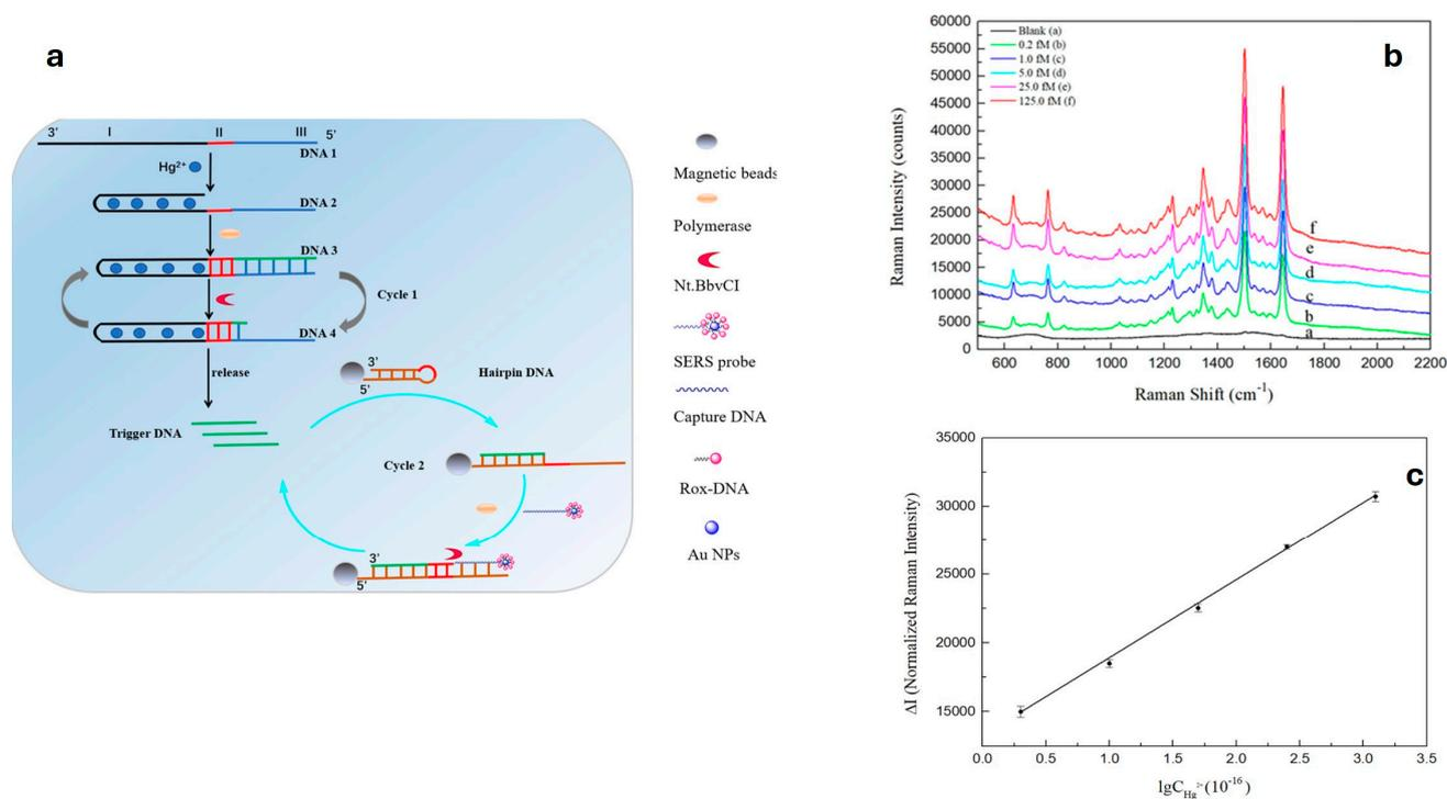
**Figure 8.** (a) Schematic diagram of SERS aptasensor based on dual recycling amplification for trace  $\text{Hg}^{2+}$  detection; (b) SERS spectra under different concentrations of  $\text{Hg}^{2+}$ ; (c) linear relationship between Raman intensity and different mercury ion concentrations. Reprinted from reference [88] with permission from Elsevier.
