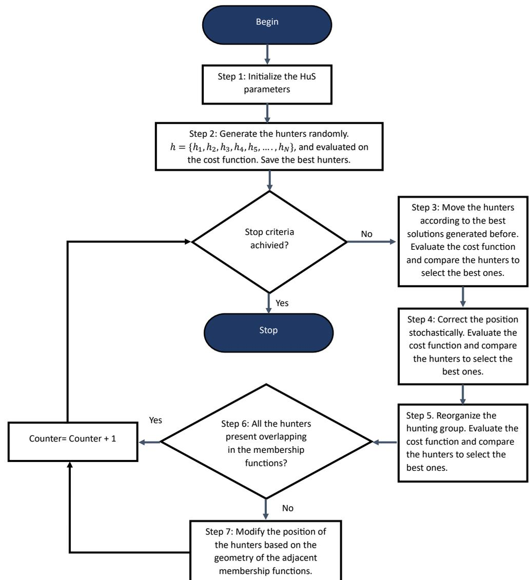
**Figure 8.** Hunting search modified to ensure overlapping of the membership functions.
