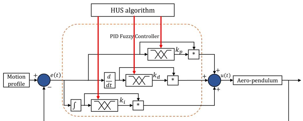
**Figure 5.** Hunting search algorithm-based adaptive PID fuzzy tracking controller proposal.
