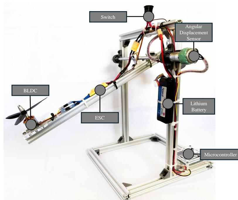
Figure 1. Aero-pendulum system.
