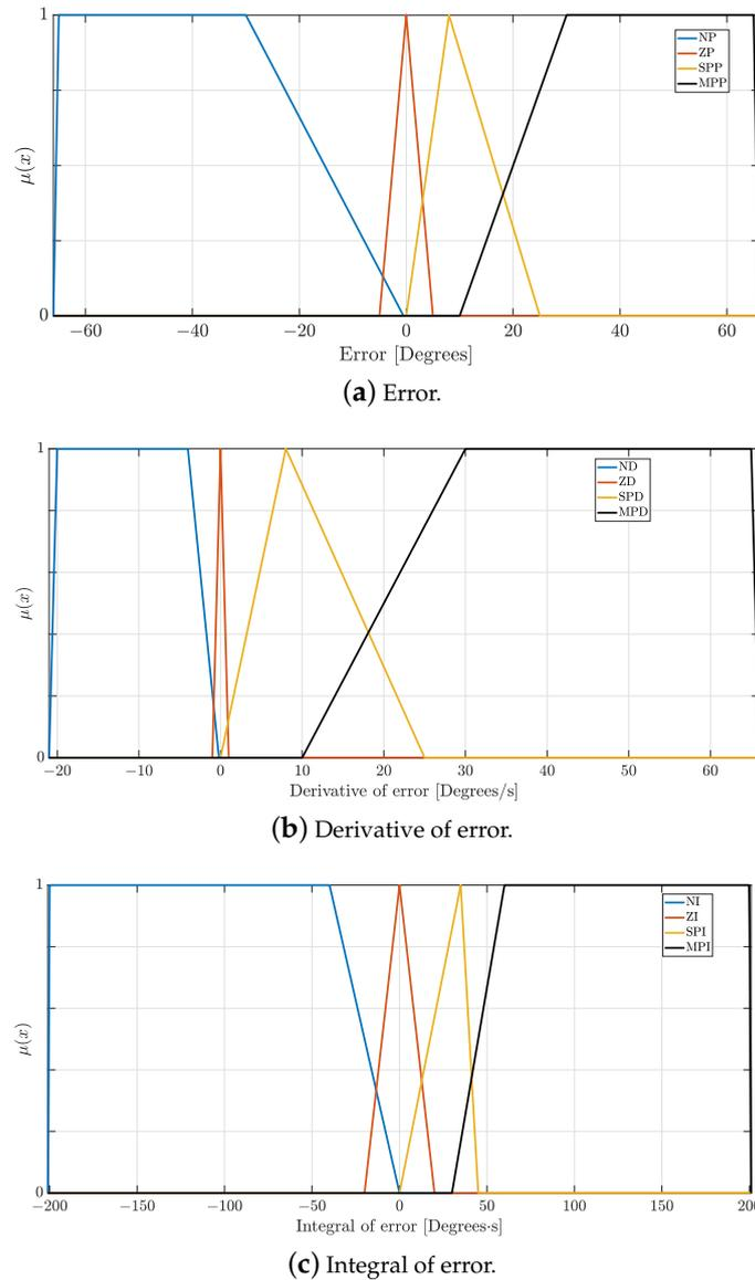
**Figure 10.** Non-optimized input linguistic variables (a) error, (b) derivative of error, and (c) integral of error.
