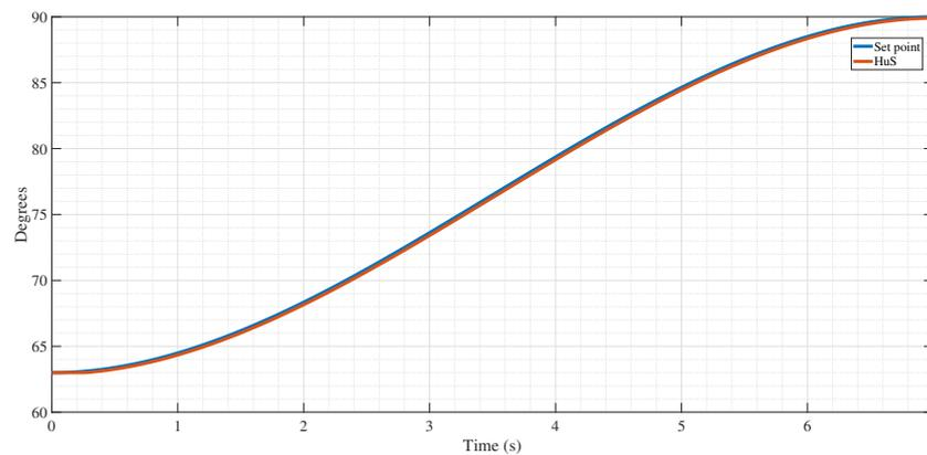
**Figure 13.** Reference vs. fuzzy controller optimized by HuS algorithm.
