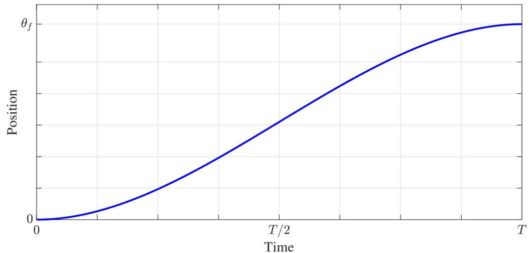
**Figure 4.** Position in a parabolic motion profile.
