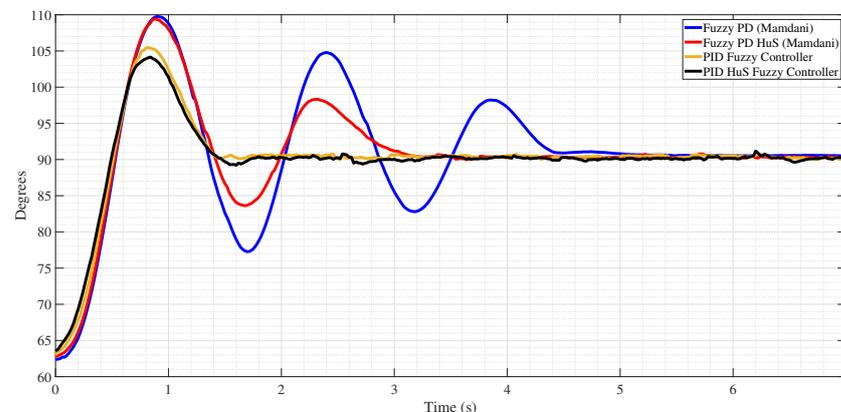
**Figure 19.** Step comparison of non-adaptive and adaptive fuzzy controllers.
