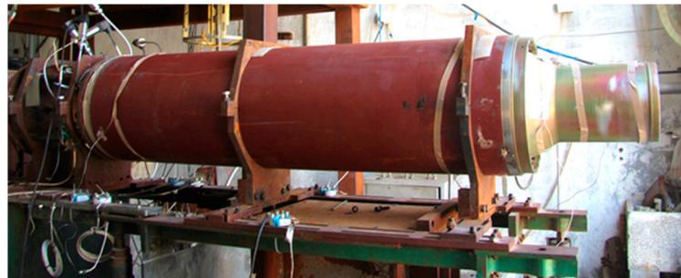
Figure 5. Photograph of the hybrid rocket motor before the test.
