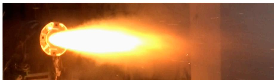
**Figure 12.** Hybrid rocket motor 200-s ground firing test.
