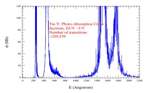
**Figure 13.** Photoabsorption cross-sections ( $\sigma$ ) of Tm V in the energy range of EUV to UV. It demonstrates multiple broad structures from the EUV to the UV wavelength range, with the widest one being in the range of 1400–1900 Å with a dip at around 1650 Å.
