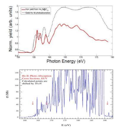
**Figure 1.** Photoabsorption cross-sections ( $\sigma$ ) of Ho II. Top: Experimental photoabsorption spectrum (black dashed curve) of Ho [23]. Bottom: Predicted spectrum of Ho II from the present work. The predicted
