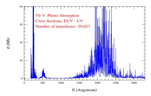
**Figure 18.** Photoabsorption cross-sections ( $\sigma$ ) of Yb V in the energy range of E to EUV to UV. It has two broad features dominated by strong lines: one in the EUV region followed by a lower peak structure and a broader absorption bump in the wavelength region of 1600–2500 Å.
