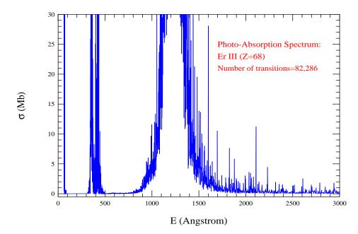
**Figure 7.** Photoabsorption cross-sections ( $\sigma$ ) of Er III demonstrating three regions of high peak strong lines from X-ray to UV regions: the first one is in the narrow X-ray region (around 80 Å), one is a relatively narrow region in the EUV range (300–500 Å), and one is a relatively large broad spectral region in the UV range (900–1700 Å).
