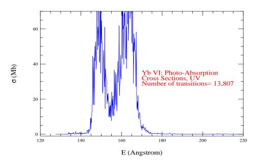
**Figure 19.** Photoabsorption cross-sections ( $\sigma$ ) of Yb VI in the energy range of UV. It has two absorption bumps next to each other in the energy range of 145–170 Å.
