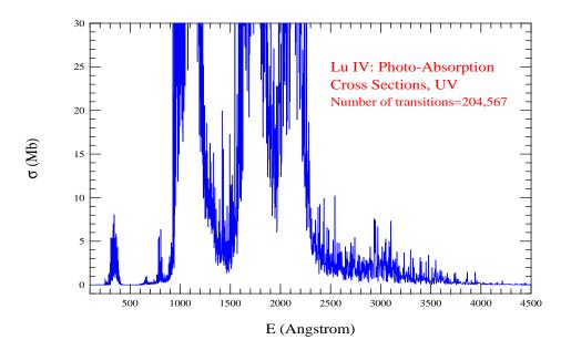
**Figure 23.** Photoabsorption cross-sections ( $\sigma$ ) of Lu IV in the energy range of UV, showing multiple absorption bumps in the UV region.
