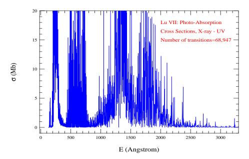
**Figure 26.** Photoabsorption cross-sections ( $\sigma$ ) of Lu VII with prominent absorption lines in the energy range of EUV–UV. The spectrum shows multiple broad absorption energy bumps in the energy region. The prominence of strong lines in the absorption bumps, one from 150 Å in the X-ray range to 350 Å in the EUV range and one from 400–800 Å in UV, can be seen. Two absorption bumps exist next to each, covering a energy width of about 1000 to 2200 Å.
