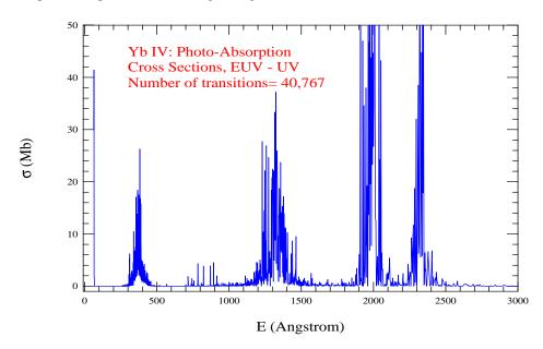
**Figure 17.** Photoabsorption cross-sections ( $\sigma$ ) of Yb IV in the energy range of E to EUV to UV, exhibiting multiple regions of strong lines.
