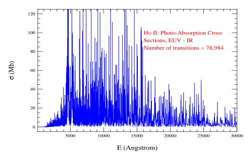
**Figure 3.** Photoabsorption cross-sections ( $\sigma$ ) of Ho II demonstrating broad spectral feature in the UV wavelength region.
