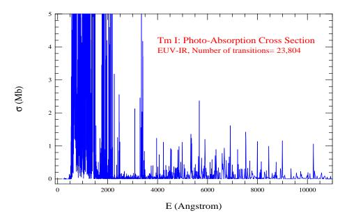
**Figure 9.** Photoabsorption cross-sections ( $\sigma$ ) of Tm I demonstrating three regions of high peak strong lines: one in the EUV region of 500–1500 Å, the second one in 1700–2500 Å, and the third one in the narrow band around 3400 Å. Noticeable lines become more sparse with larger wavelengths.
