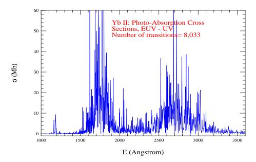
**Figure 15.** Photoabsorption cross-sections ( $\sigma$ ) of Yb II with dominating strong lines in the energy range of EUV–UV. The spectrum shows two broad features, one in the wavelength range of 1500–2100 Å and another one in 2500–3100 Å.
