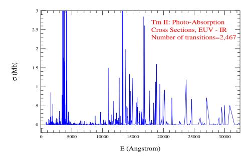
**Figure 10.** Photoabsorption cross-sections ( $\sigma$ ) of Tm II demonstrating the visible presence of strong lines in the UV and IR regions and almost no strong lines in the optical (4000–7000 Å) region. Compared to other lanthanides discussed here, this ion has a smaller number of transitions and a relatively wider broad feature exists in the IR region.
