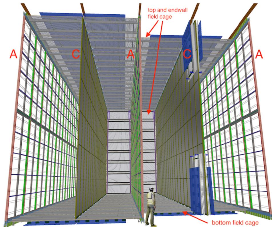
**Figure 2.** The DUNE Horizontal Drift liquid argon TPC, showing the alternating 58.2 m long (into the page), 12.0 m high anode (A) and cathode (C) planes, as well as the field cage (FC) that surrounds the drift regions between the anode and cathode planes. For the sake of illustration, on the right-hand cathode plane, the foremost portion of the FC is shown in its undeployed (folded) state. Reproduced from [46] under the CC BY 4.0 license.
