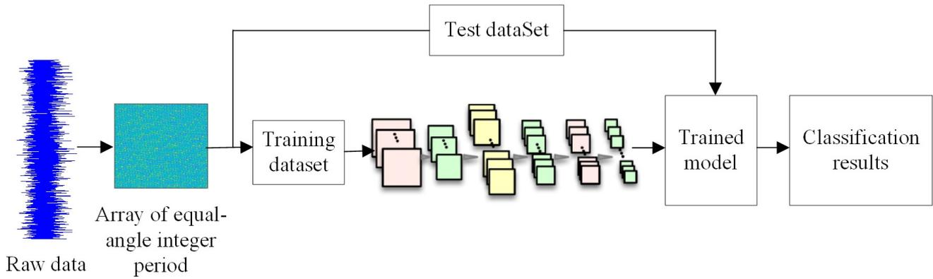
Figure 3. Program of fault diagnosis using CNN and uniform angle sampling.
