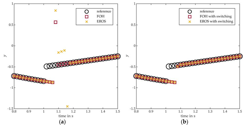
**Figure 6.** Behavior of coupling algorithms FOH and EROS in the case where a discontinuity occurs in the coupling signal for a latency of  $k = 3$  macro steps: (a) without discontinuity detection; (b) with discontinuity detection and algorithm switching.
