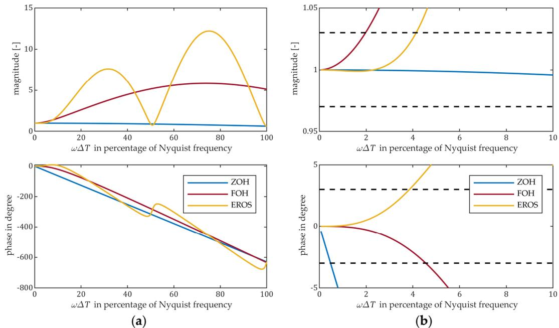
**Figure 3.** Bode plot of the coupling process of RVPs for an exemplary latency of  $k = 3$ , normalized to the frequency with respect to the macro step as a percentage of the Nyquist frequency (compare to [37] for non-iterative co-simulation) for the coupling algorithms zero-order-hold (ZOH), first-order-hold (FOH), and error space extrapolation (EROS): (a) overview; (b) focus on low frequencies. Magnitude and phase limits as introduced by the authors of [37] are shown as a dashed line.
