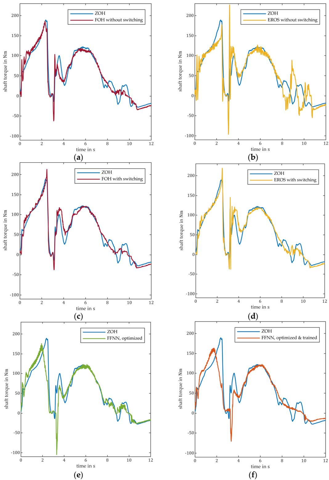
**Figure 10.** Latency-compensated shaft torque signal of the RVP when using different coupling algorithms, as compared to the naïve ZOH method: (a,b) FOH and EROS, without switching the algorithm; (c,d) FOH and EROS with switching the algorithm after a detected discontinuity; (e) FFNN optimized using the method from Section 2.4.2; (f) FFNN initialized, like the FFNN in (e) that was trained online during a previous run of the RVP.
