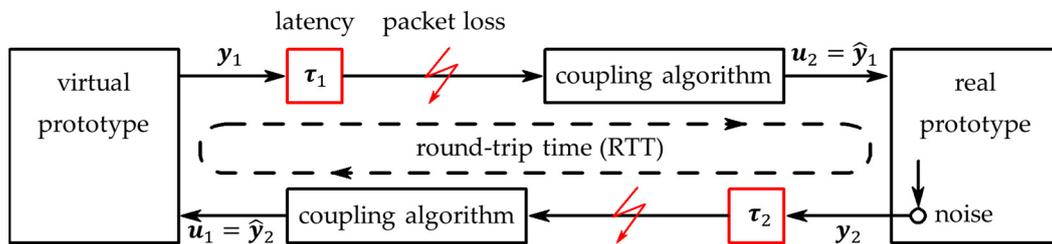
**Figure 1.** Schematic representation of a real-virtual prototype (RVP), consisting of one real and one virtual prototype, with a focus on the coupling faults during data exchange due to network effects, marked in red. Packet loss is indicated by the red flash. Based on [28].
