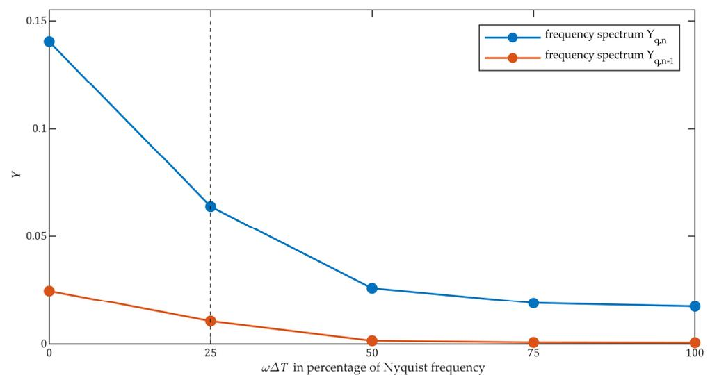
**Figure 5.** Resulting frequency spectrum for the yellow signal segment from Figure 4.  $Y_{q,n}$  represents the frequency spectrum of the current macro step, where a discontinuity occurs, while  $Y_{q,n-1}$  represents the spectrum from the previous macro step, where no discontinuity has occurred.
