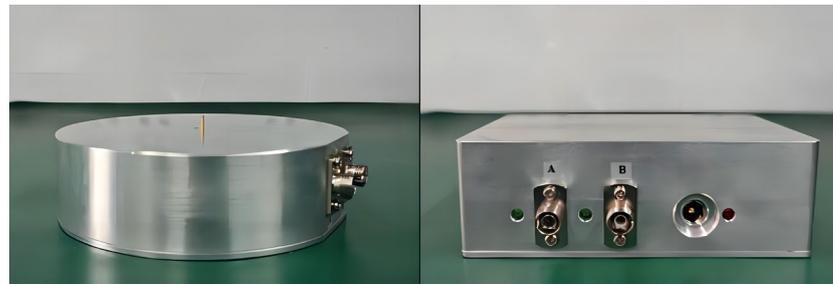
**Figure 4.** Pulsed electric-field probe and photoelectric converter.
